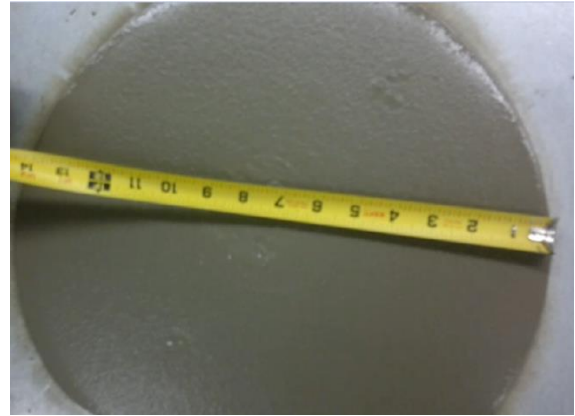
Fig. E.2 Inadequate Workability with 3 Quarts Water per 50 lb of Grout (Left); Improved Workability with 3 Quarts Water and 40 ml Superplasticizer per 50 lb Grout (Right)
