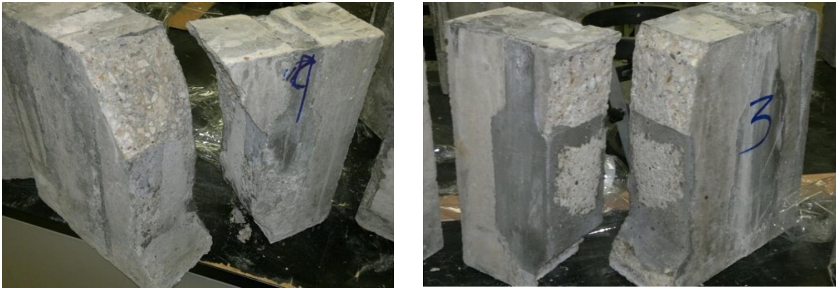
Fig. D.13 Failure Mode C - Failure in UHPG with Cement Slurry and Sandblasted Surface through Concrete and Grout Interface
