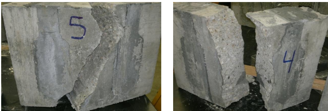
Fig. D.14 Failure Mode C - Failure through Concrete in Specimens with UHP Grout with Sandblasted Surface
