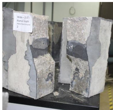
Fig. D.10 Failure Mode B in Polymer Grout, Wide-Partial Depth Key Way
