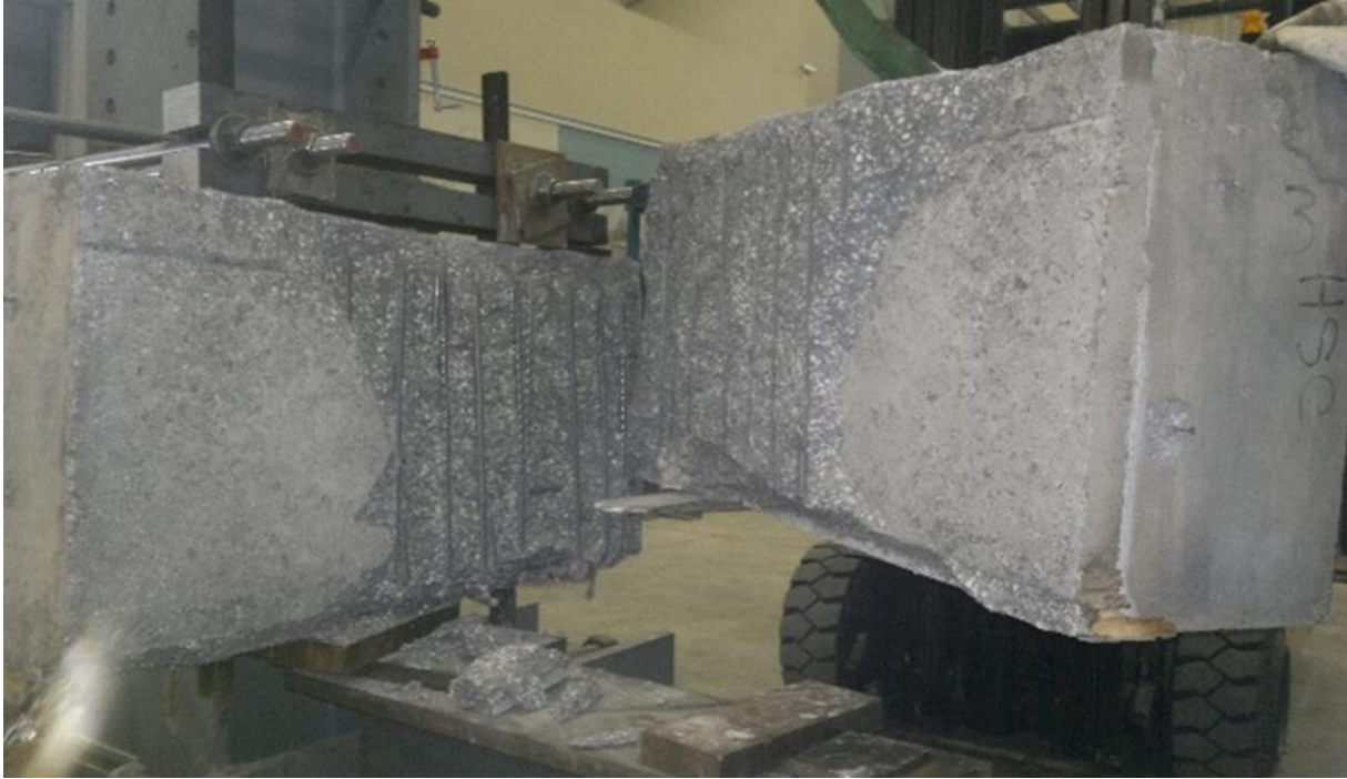
Fig. H.17 Failure of Specimens with HSC Grout
