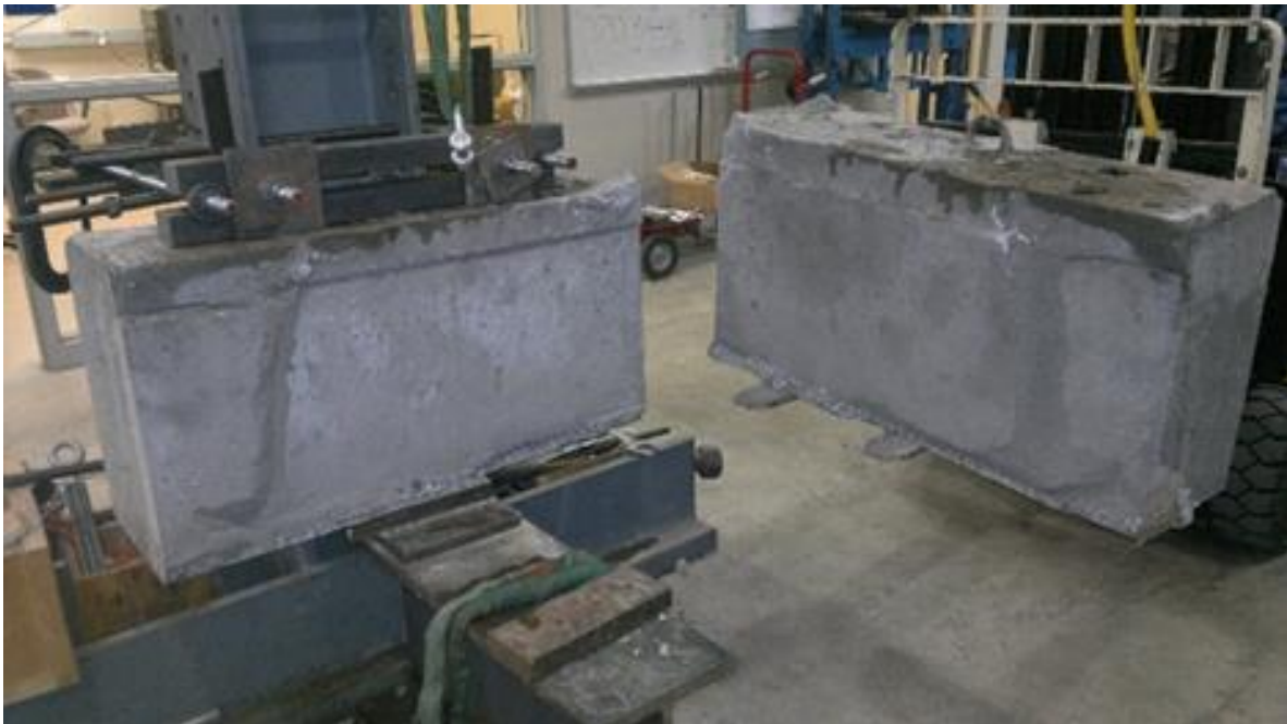
Fig. H.20 Failure of Specimens with ODOT-approved Grout
