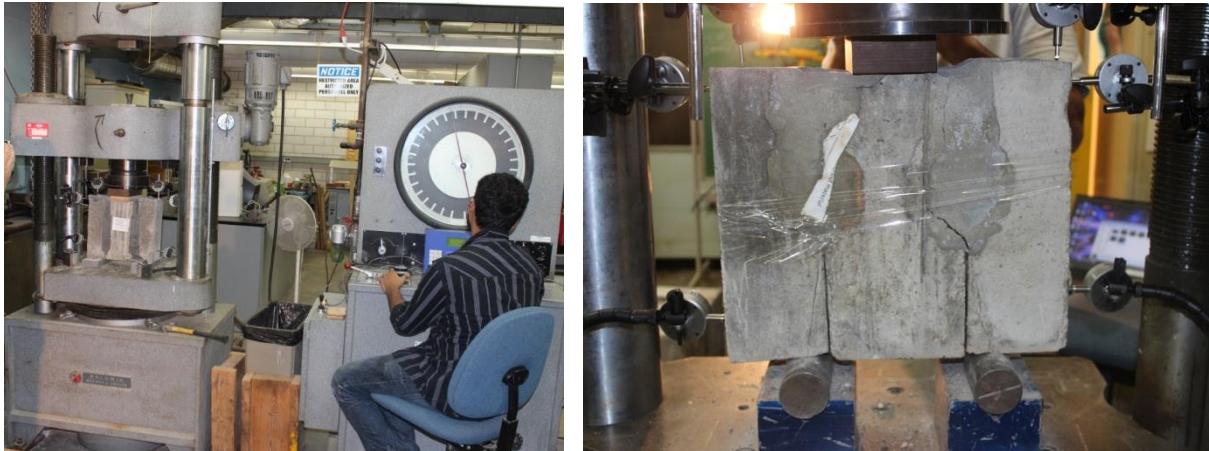
Fig. D.4 Hydraulic Test Machine (left) – Test Specimen and Setup (right)
