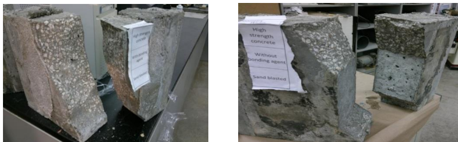
Fig. D.12 Failure Mode C - Failure in HSC Grout with Bonding Agent and Sandblasted Surface (Left); Failure in HSC Grout without Bonding Agent and With Sandblasted Surface (Right)
