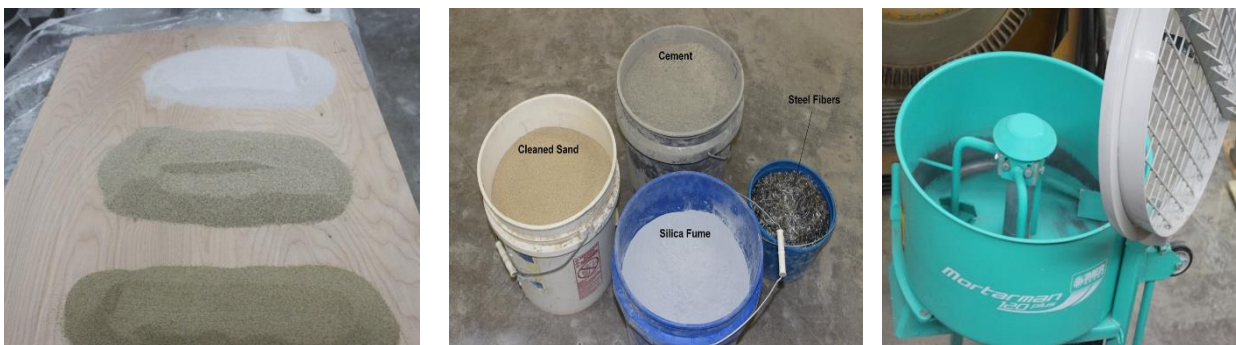
Fig E.3 Mix Ingredient and High Shear Mixer
