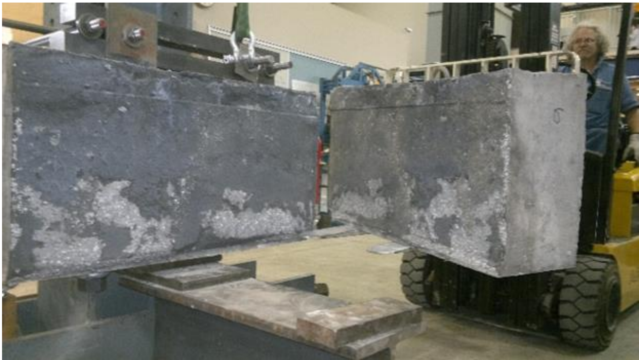
Fig. H.18 Failure of Specimens with Polymer Grout
