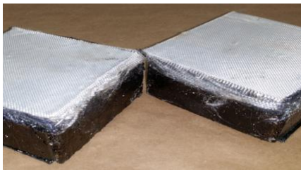
Fig. B.10 Ultimate Differential Deflection Failure Modes: Full Rupture ( left ) and Partial Rupture ( right )
