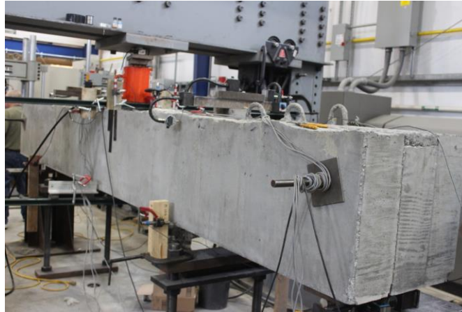
Fig. F.7 Test Setup for Beam Assemblies
