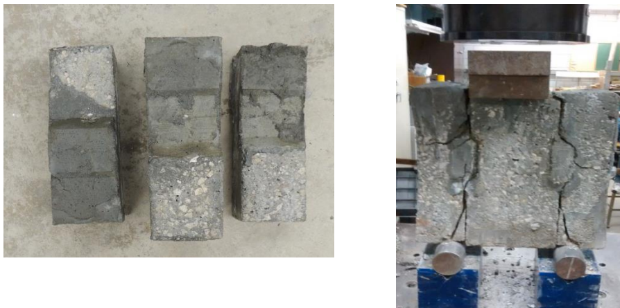
Fig. D.3 Typical Failure Mode, Specimens without Ties (left) Specimen with Tie Rod (right)
