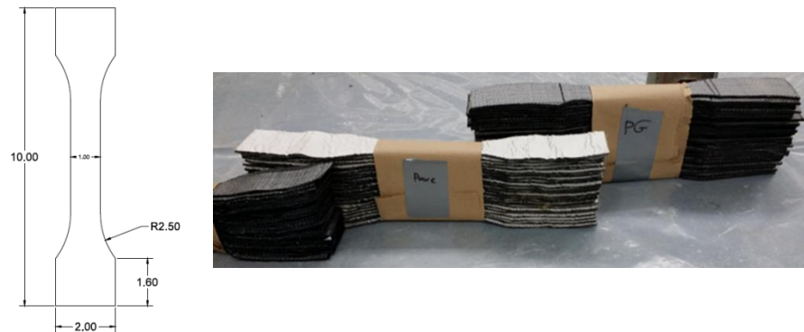
Fig. B.1 Typical Tensile and Elongation Test Specimen Dimensions (inches)
