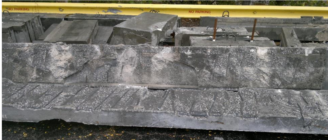
Fig. F.21 Set#7 Separation of Concrete Cover After Testing
