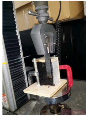
Fig. B.6 Adhesion Test Details
