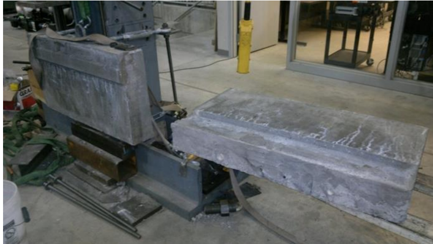
Fig. H.10 Failure of the Test Specimen with Kuhlman Grout and Partial Depth Keyway
