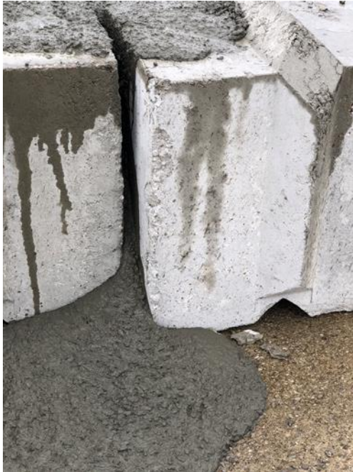
Fig. J.3 Trial Grout – Note the Spread of the Grout (Left); the Grout Consistency (Right)
