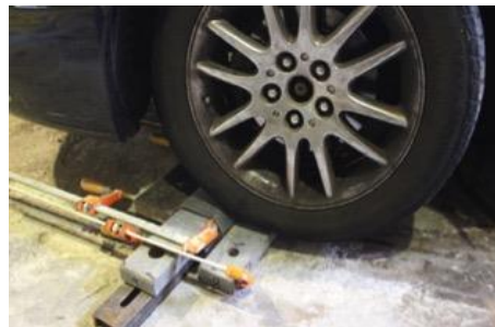
Fig. B.18 Membrane Subjected to Wheel Loading (1,200 lb)
