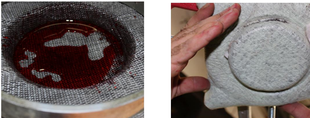
Fig. B.13 Top ( left ) and Bottom ( right ) Views of a Typical Test Specimen after the Test, Showing no Leakage at the Bottom
