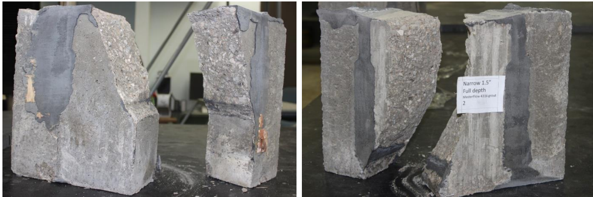
Fig. D.15 Failure Mode C - Failure in Polymer Grout: Narrow-Partial Depth Key Way (Left), Full Depth Key Way (Right)
