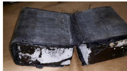
Fig. B.10 Ultimate Differential Deflection Failure Modes: Full Rupture ( left ) and Partial Rupture ( right )
