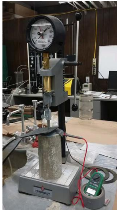
Fig. B.16 Punching Test Setup
