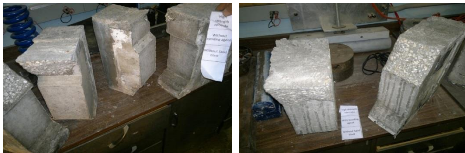
Fig. D.11 Failure Mode C - Failure in HSC Grout (Left); Failure in HSC Grout with Bonding Agent (Right)
