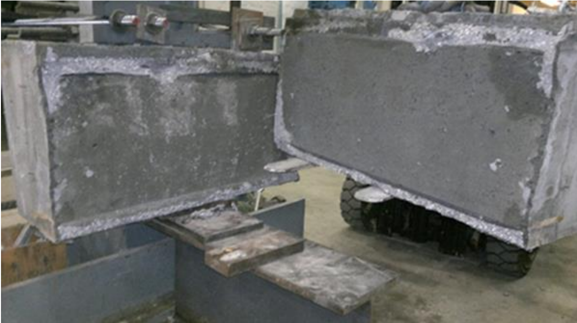
Fig. H.19 Failure of Specimens with UHPG
