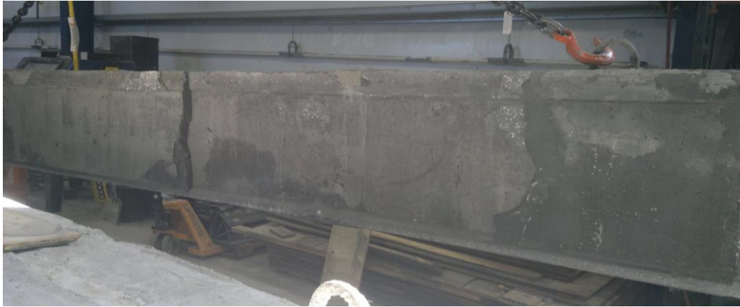
Fig. F.18 Set # 6 Middle Concrete Unit After Failure
