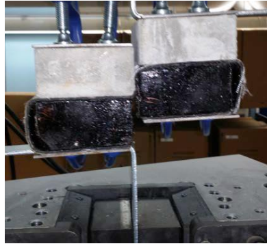
Fig. B.8 Ultimate Differential Deflection Test Details
