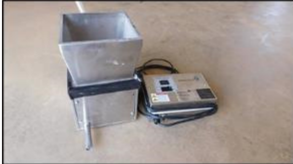
(c) Schenck Process Model 106M Material Feeder
