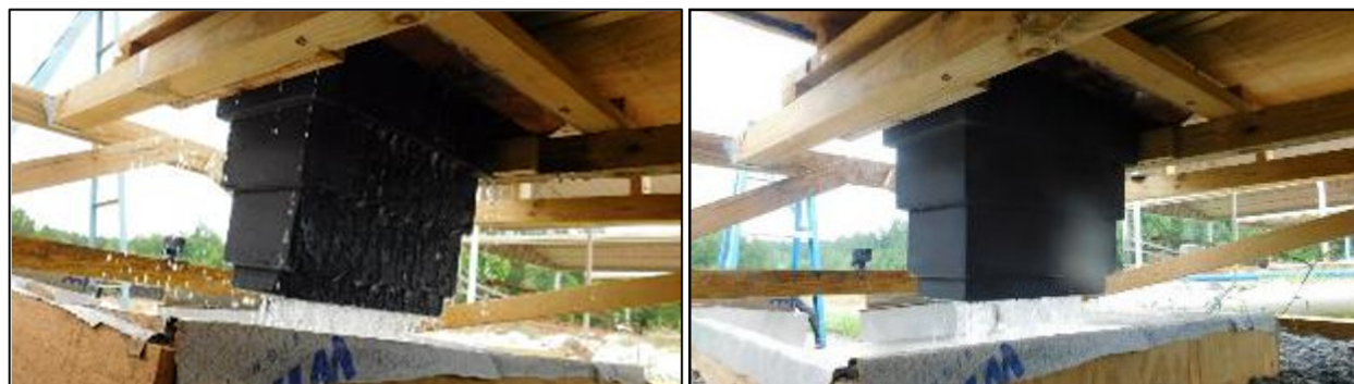
(a) sheet flow (b) direct discharge Figure 5-8: Bypass allowed between discharge methods.
