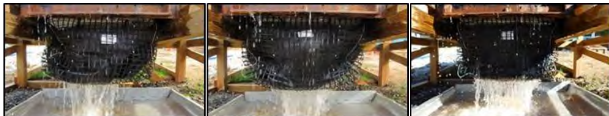
(b) direct discharge testing with OK110 silica sand
