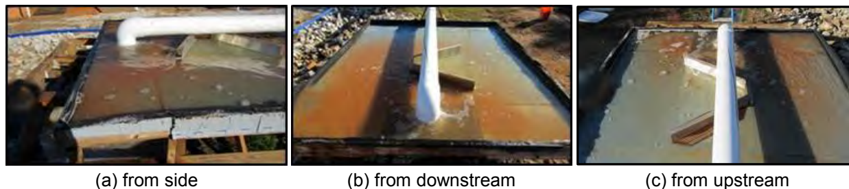
Figure C-21: Flooding during WQS high flow test using sandy loam soil under direct discharge conditions.
