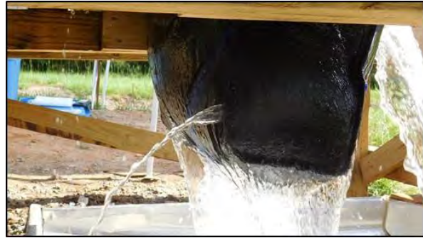
(b) direct discharge with OK110 silica sand
