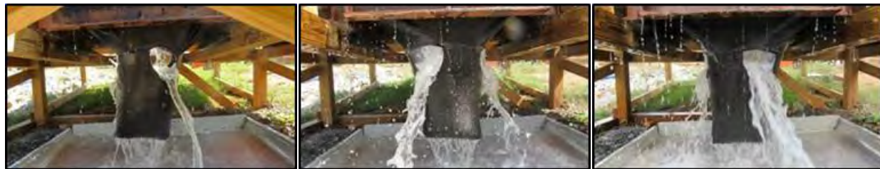
(a) sheet flow testing with OK110 silica sand
