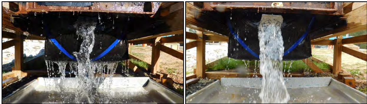
(a) L1 (b) L2 Figure C-26: Gullywasher© during longevity testing with sandy loam soil.
