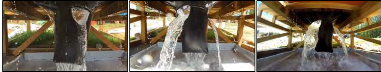
Figure C-16: Storm Sentinel® during testing using various test methods and soil types.
