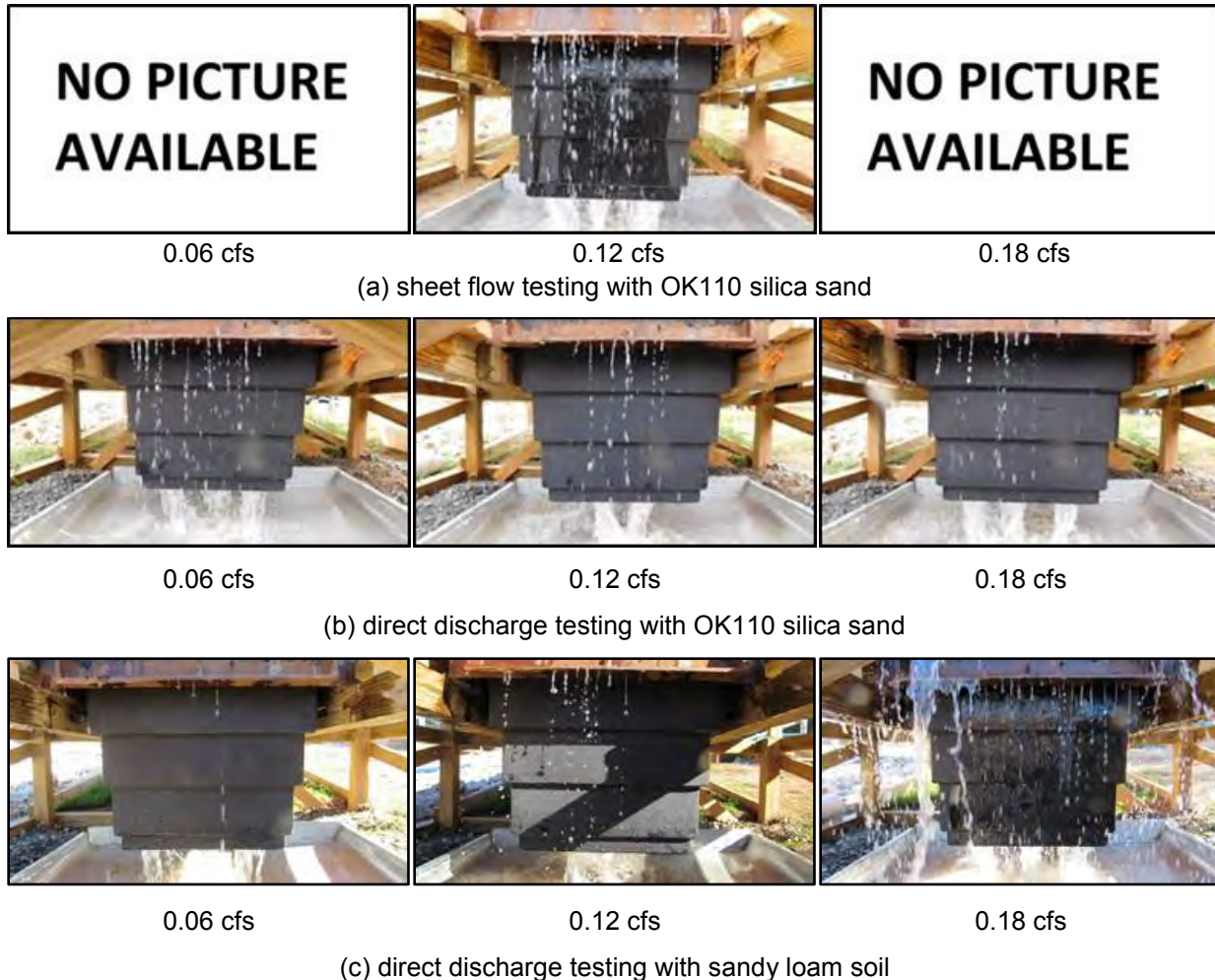
Figure C-20: WQS during testing using various test methods and soil types.
