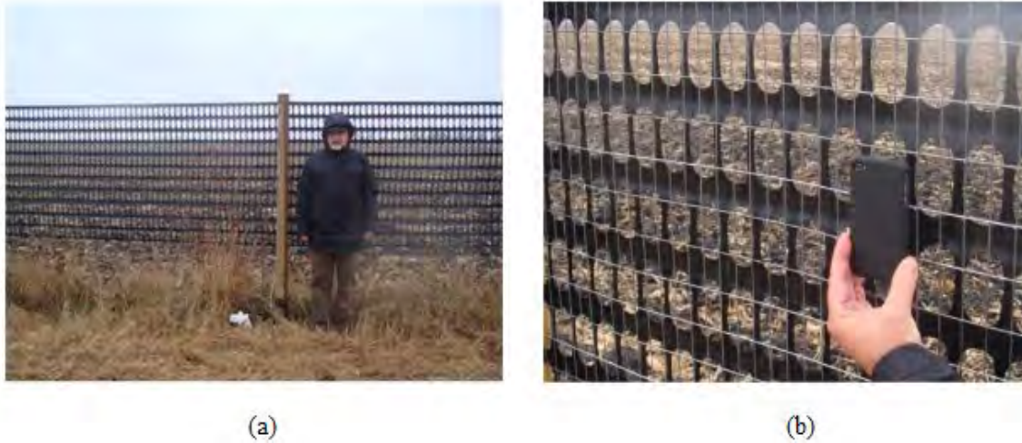
Figure 12. (a) View of one of the lightweight plastic snow fences tested at the field site (A1 fence: P=50\% , G/H=0.34 , H \approx 1.9 ); (b) Close view showing the 2 mm diameter welded wire frame used to support the plastic fence.
