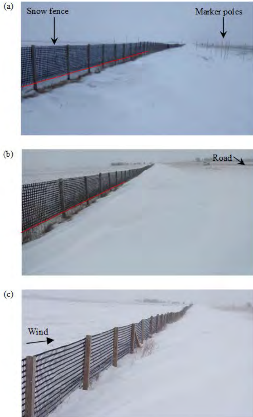
Figure 74. Views showing snow deposition close to the fence immediately after the end of the largest snow event during the second winter: a) B1 fence ( P=30\% , G/H=0.25 ; b) B2 fence ( P=30\% , G/H=0.2 ); and c) A3 fence ( P=50\% and G/H=0.08 ). The red lines indicate bottom of the fence.
