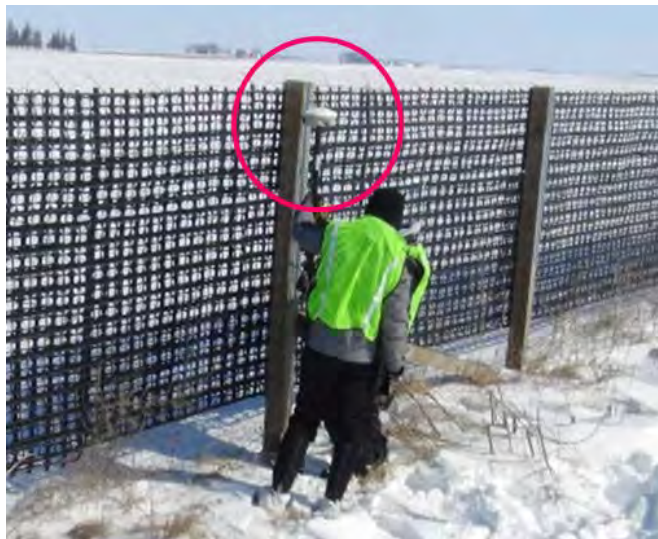
Figure 30. RTK survey conducted along the marker poles line.
