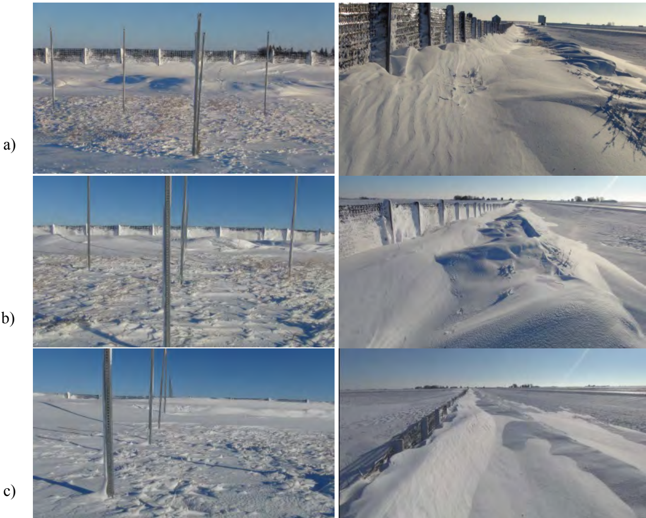
Figure 95. Views showing snow deposition close to the fence immediately after the end of the largest snow event during the third winter season: a) B1 fence ( P=30\% , G/H=0.25 ; b) B2 fence ( P=30\% , G/H=0.2 ); and c) A3 fence ( P=50\% and G/H=0.08 ).
