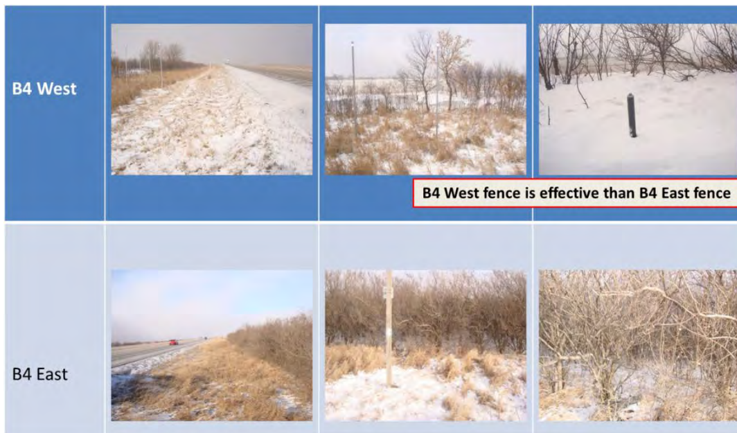
Figure 86. Snow deposition after a snow storm close to the living snow fence at west side and the living snow fence at the east side.
