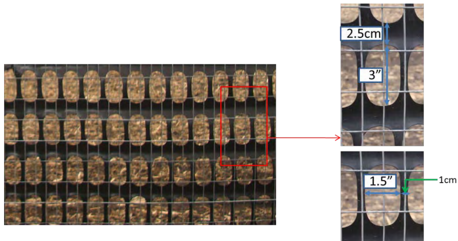
Figure 14. Detail view showing layout of plastic fence.
