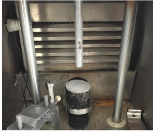
Figure 5 Ice layer rupture test (Ma et al. 2016)
