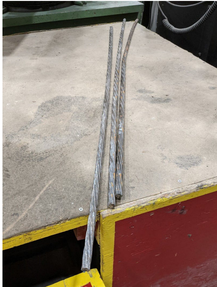
Figure 34. Steel strand samples for tensile tests
