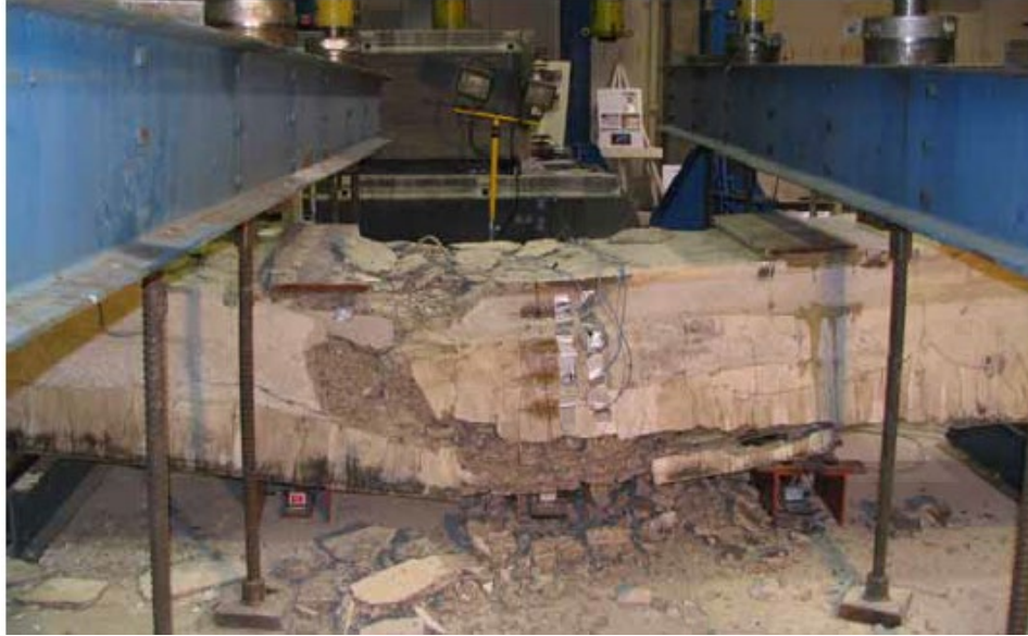
Figure 20. US 7 Beam #14 failure
