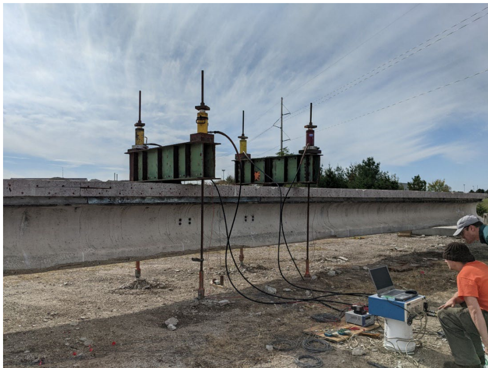
Figure 63. Girder G bending load test
