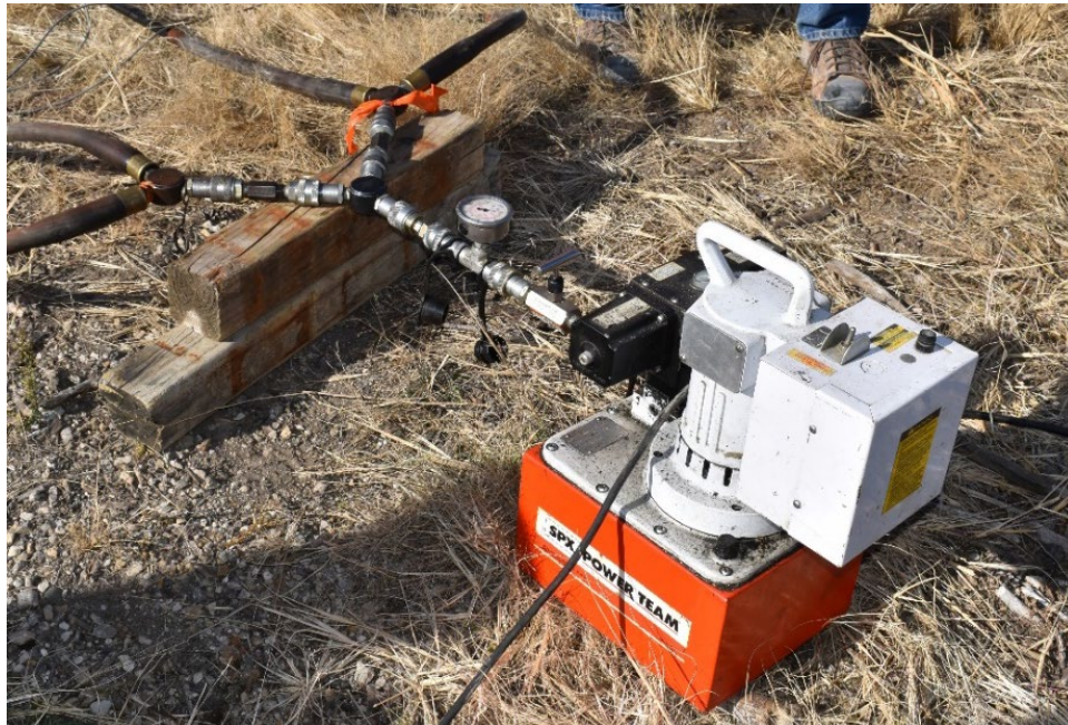
Figure 40. Hydraulic pump with four-hose manifold
