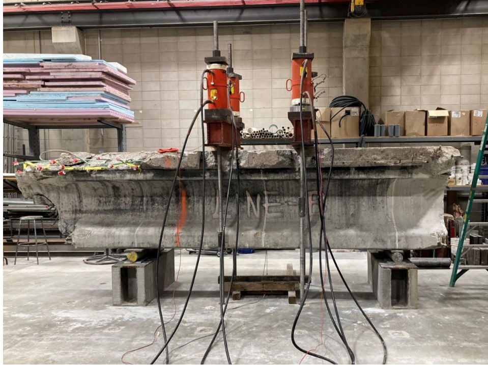
Figure 42. Girder end shear test configuration
