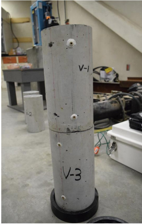
Figure 3-7. Specimens Epoxied with Gauge Plugs
