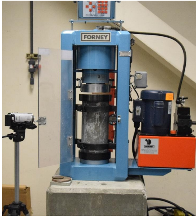
Figure 4-12. Stress-Strain Test using Forney Compression Machine & Compressometer
