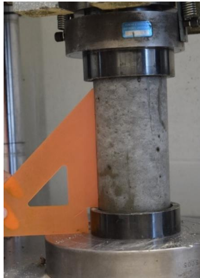
Figure 4-8. 28-Day Break Cylinder Strength Test Loading
