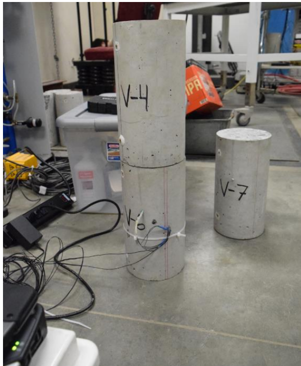
Figure 3-8. Specimens Pre-Loading Set Up with Thermistors
