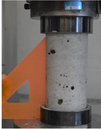
Figure 4-5. 7-Day Break Cylinder Strength Test Loading
