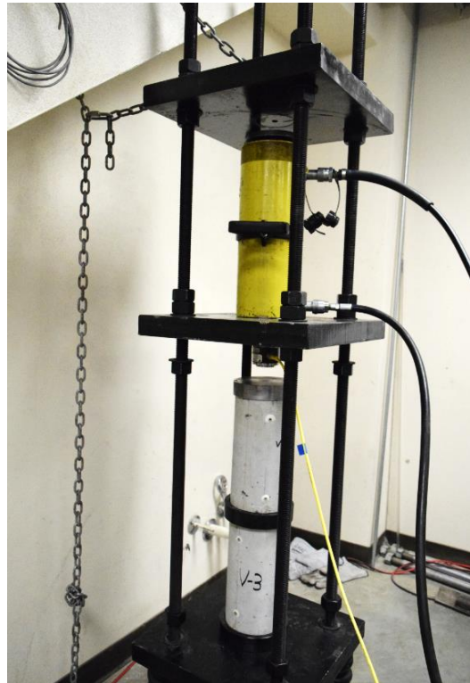
Figure 4-1. Specimens Loading Set Up Indoor Frame
