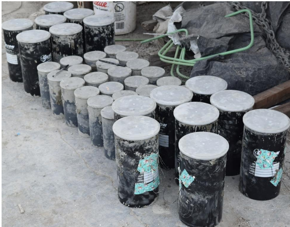
Figure 3-6. Completion of Making Concrete Cylinders in the Field
