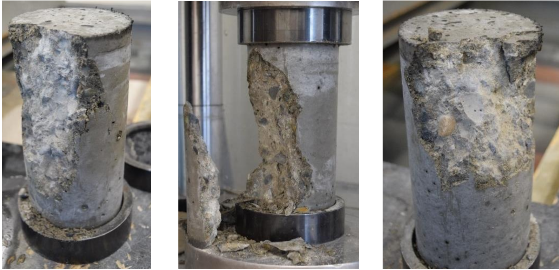
Figure 4-9. 28- Day Break Strength Test Results 1 through 3 in Frame
