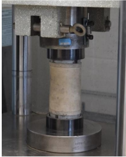
Figure 4-3. 3-Day Break Cylinder Strength Test Loading
