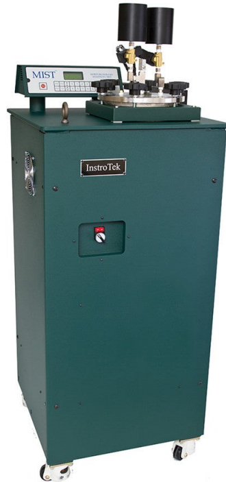
Figure 4.3: Moisture-induced sensitivity tester (MIST) equipment (InstroTek 2011)
