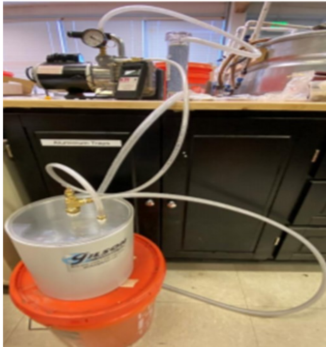
Figure 4.2: Setup used for vacuum conditioning
