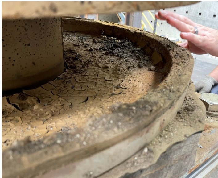
Figure 2.6. Condition of Aged Susitna 1 upon removing the seals following “as received” test.
