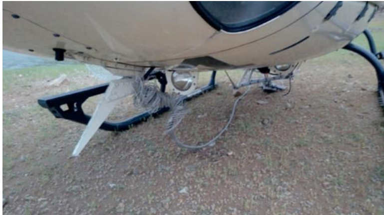
Figure 57. Wire cutter after a wire strike incident
