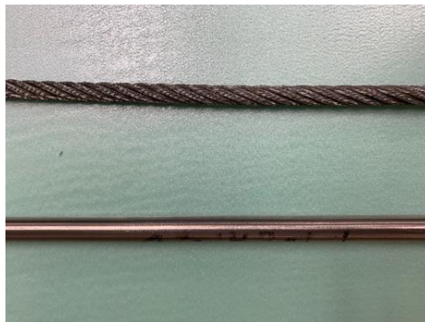
Figure 114. Picture of a stranded (top) and solid wire (bottom) both with a diameter of \sim 12.5 mm
