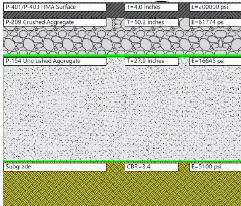
Figure 7. FAARFIELD Design Based on AC 150/5320-6G Using Design Traffic at Nome Airport
