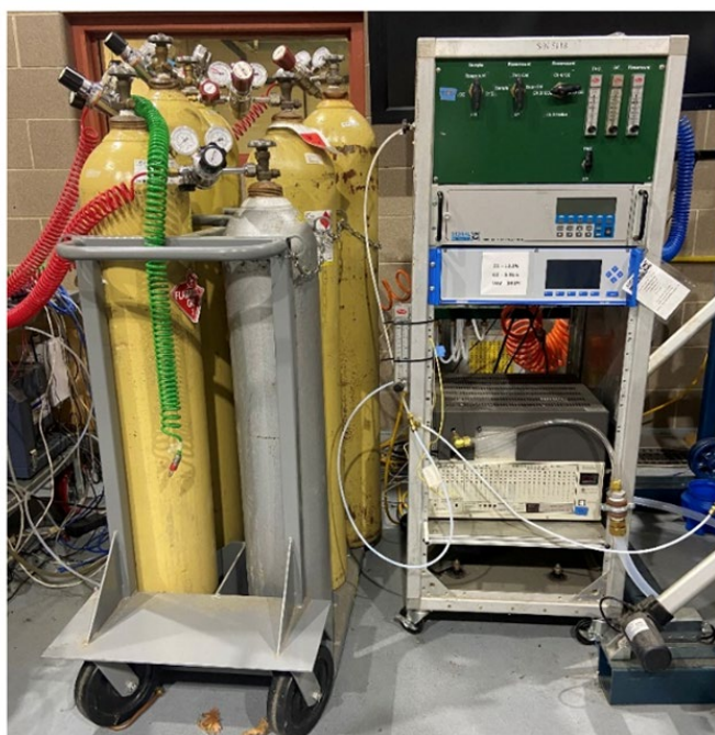
Figure 4. Gas analyzers and calibration gases
