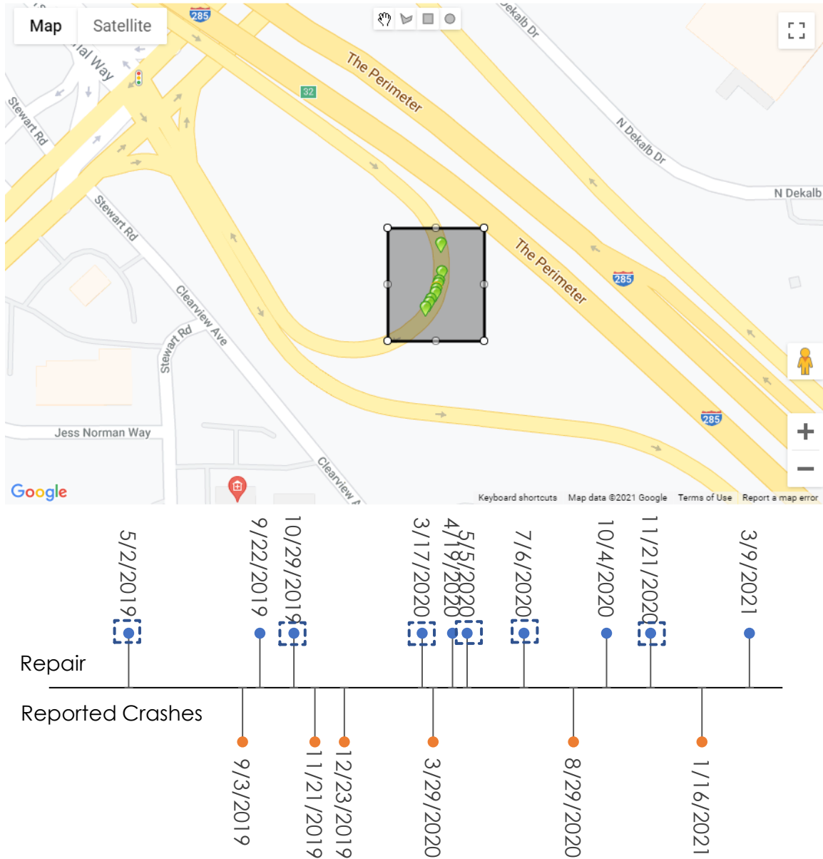
Figure 6. Map. Crash and maintenance records at the Exit 32 ramp on I-285EB.
