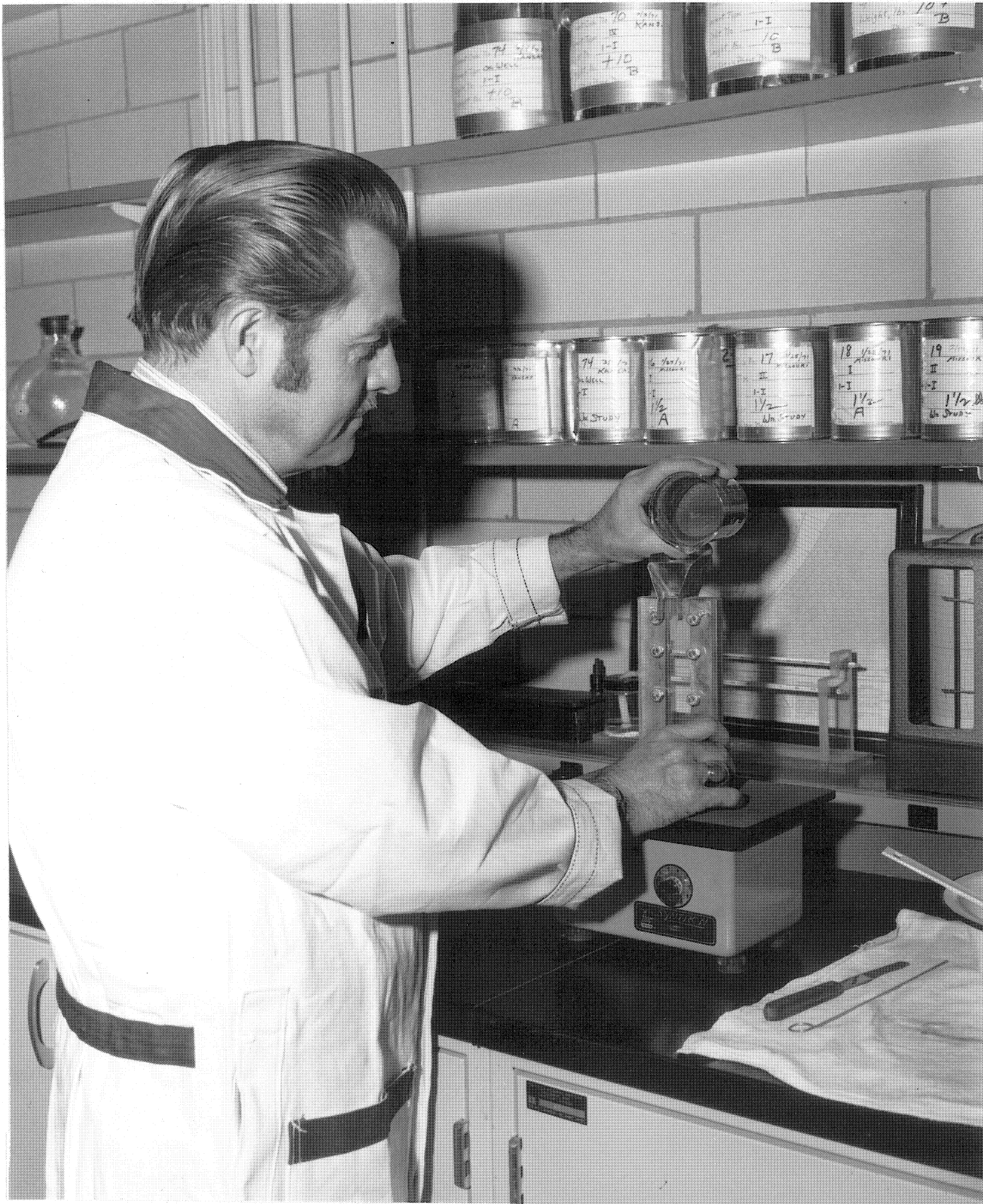
FIGURE 1. PREPARATION OF CEMENT PASTE SLAB SPECIMENS
