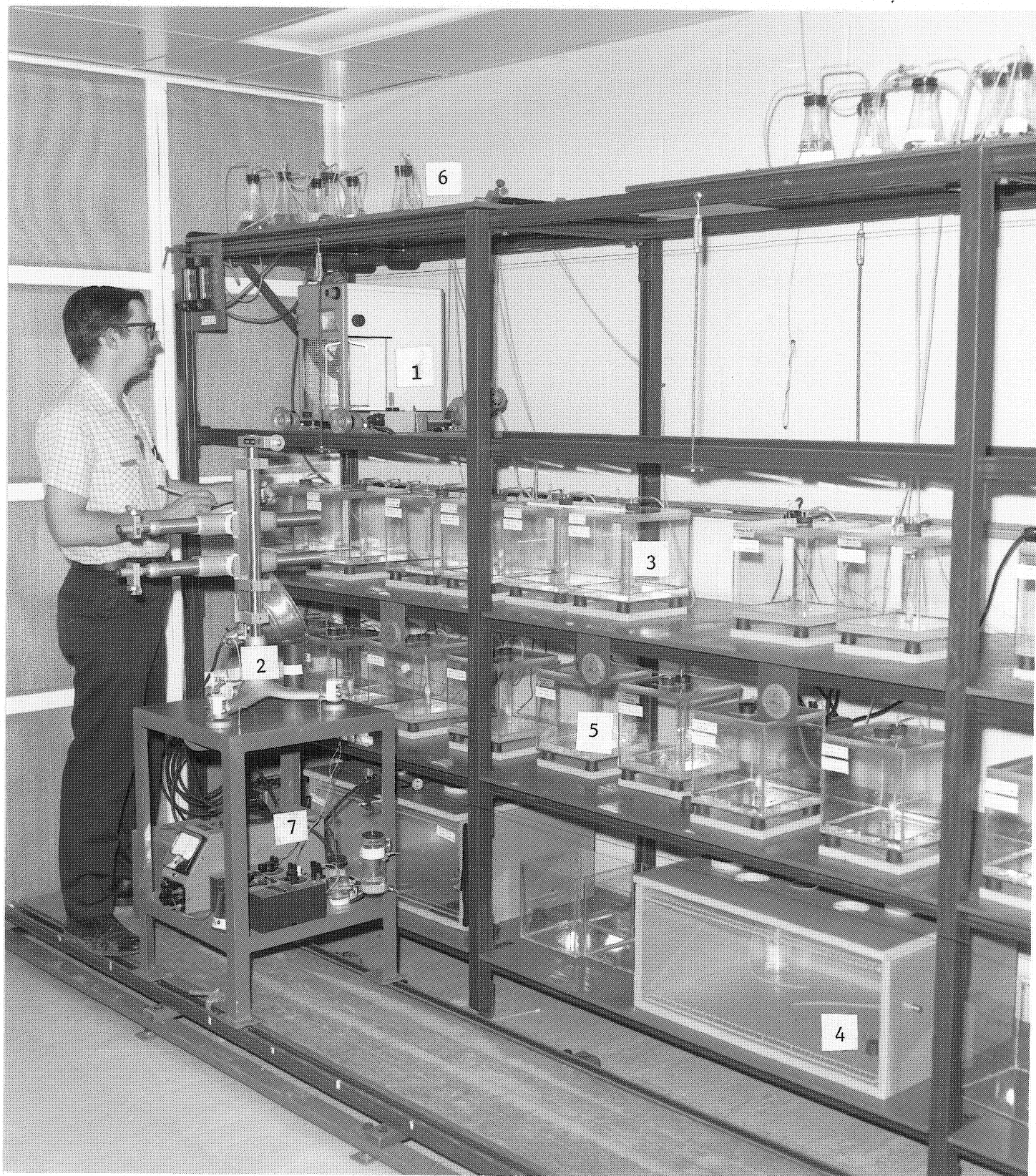
FIGURE 2. EXPERIMENTAL APPARATUS USED IN THE MEASUREMENT OF MOISTURE MIGRATION IN HARDENED CEMENT PASTES SHOWING (1) ANALYTICAL BALANCE ON MOVABLE PLATFORM, (2) OPTICAL EXTENSOMETER ON MOVABLE PLATFORM, (3) ENVIRONMENTAL CHAMBERS CONTAINING SPECIMENS, (4) OVENS FOR MAINTAINING CHAMBERS AT 100 F, (5) ELECTRICAL TIMERS, (6) PURGE GAS TRAIN, (7) MONFORE RELATIVE HUMIDITY INDICATOR
