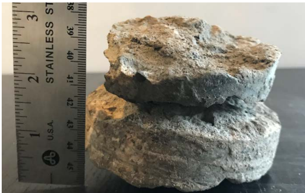
Figure A-14. Site #8, RM-3 Core #1—concrete pavement core pieces (State Route 66 SB, Stevens Point).
