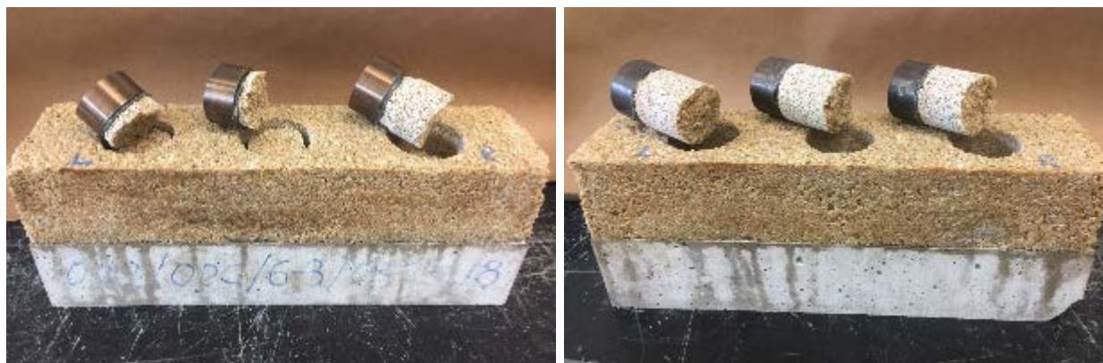
Figure 4-12. Failures observed after pull-off testing at 23 °C (left, shallow failures) and -10 °C (right, deep failures).
