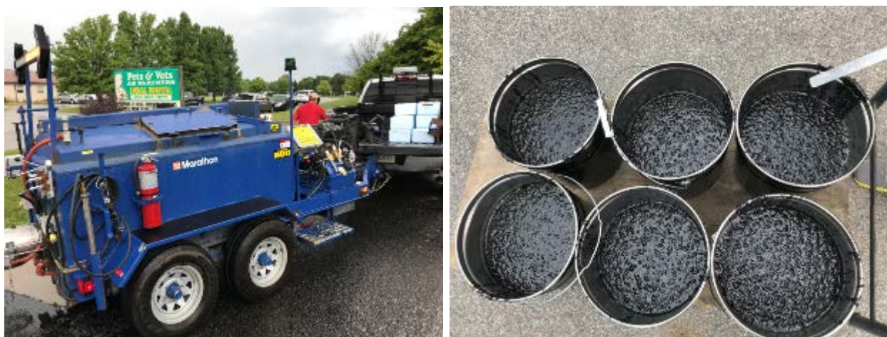
Figure 4-5. RM-5 mixing equipment (left) and prepared mixtures stored in steel pails for specimen preparation (right).
