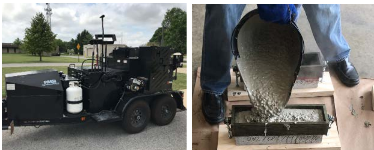
Figure 4-3. RM-4 mixing equipment (left) and specimen preparation (right).
