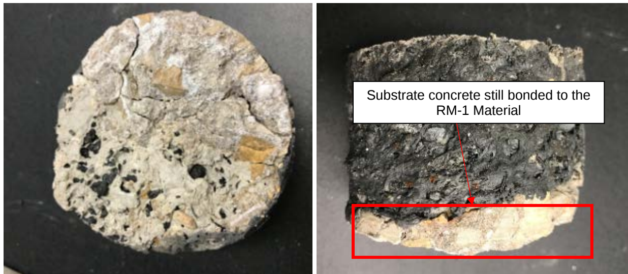
Figure 3-6. Close-up view of the bottom (left) and side (right) of the debonded portion from core #2.
