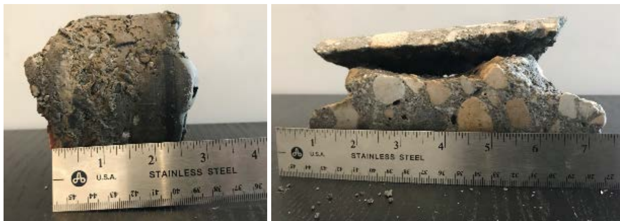
Figure 3-17. RM-4 core from Site #9 (left) and pieces of underlying concrete pavement extracted from the core hole (right).
