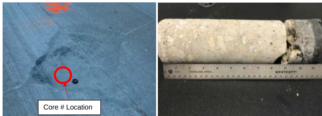
Figure 3-3. RM-1 core location #1 (left) and extracted core #1 (right).
