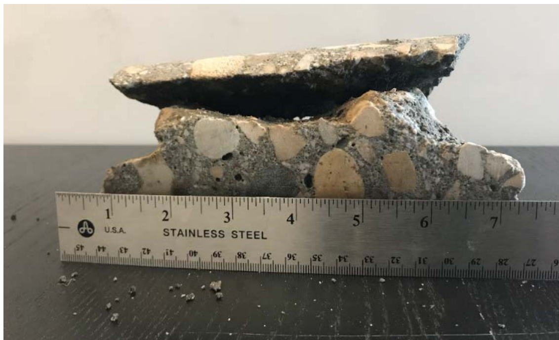
Figure A-16. Site #9, RM-4 Core #1—concrete portion (Washington St., Grafton).
