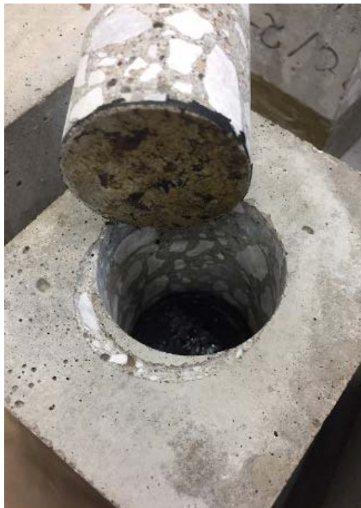
Figure 4-11. Specimens for bond testing prepared by coring through the concrete.
