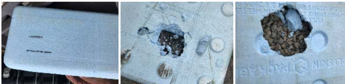
Figure 4-4. RM-5 material package (left) with binder on one side (center), and aggregates on the other (right).
