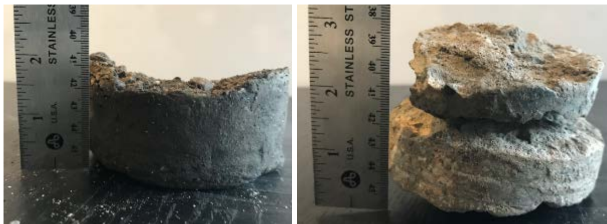
Figure 3-15. RM-3 core from Site #8 (left) and pieces of underlying concrete pavement extracted from the core hole (right).
