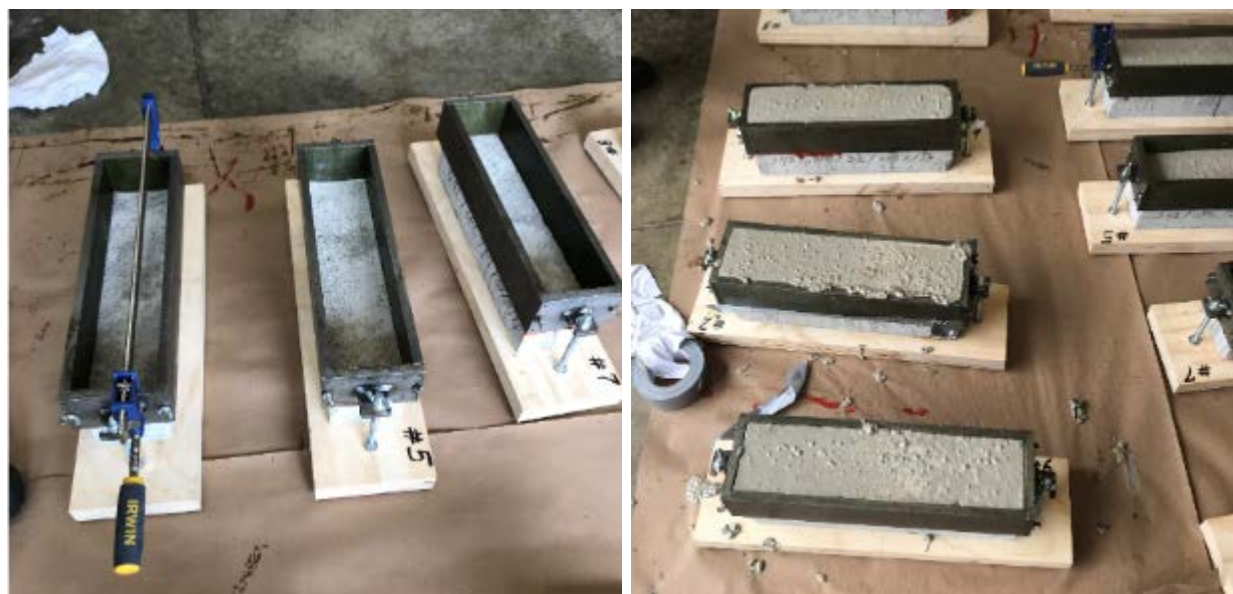
Figure 4-6. Substrate concrete beams prepared for bond testing (left) and repair material cast on top of substrate concrete beams (right)
