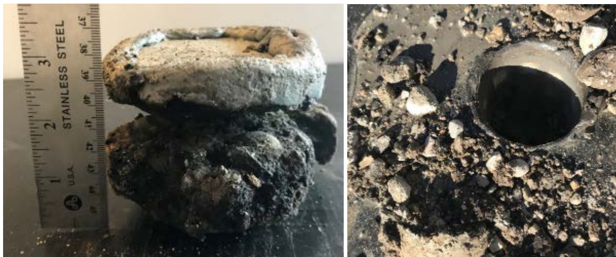
Figure 3-14. RM-3 core from Site #5 (left) and remains of underlying concrete pavement extracted from the core hole (right).
