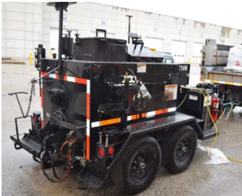
Figure 3-20. Mixing equipment used for RM-3 and RM-4.
