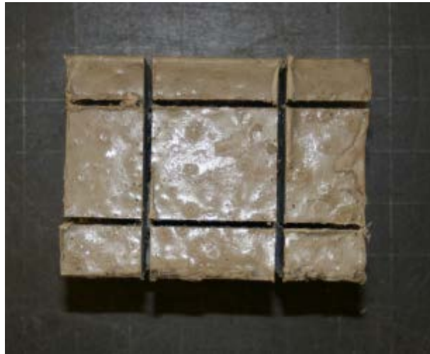
Figure 4-9. Alternate approach used to prepare specimens for bond testing.
