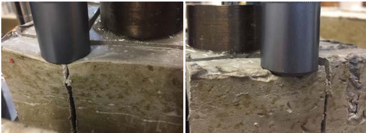
Figure 4-10. RM-4 specimens being crushed by the bond testing equipment at 23°C.
