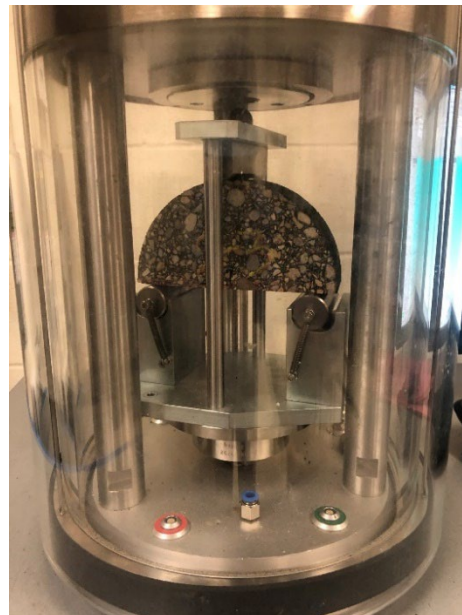
Figure 7.1: SCB Test Setup
