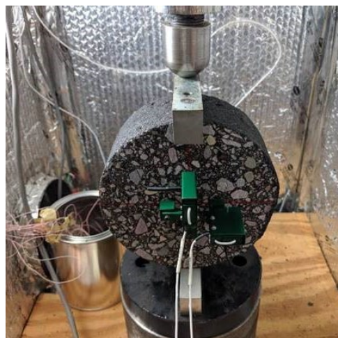
Measuring dynamic modulus of asphalt concrete in indirect tensile mode
