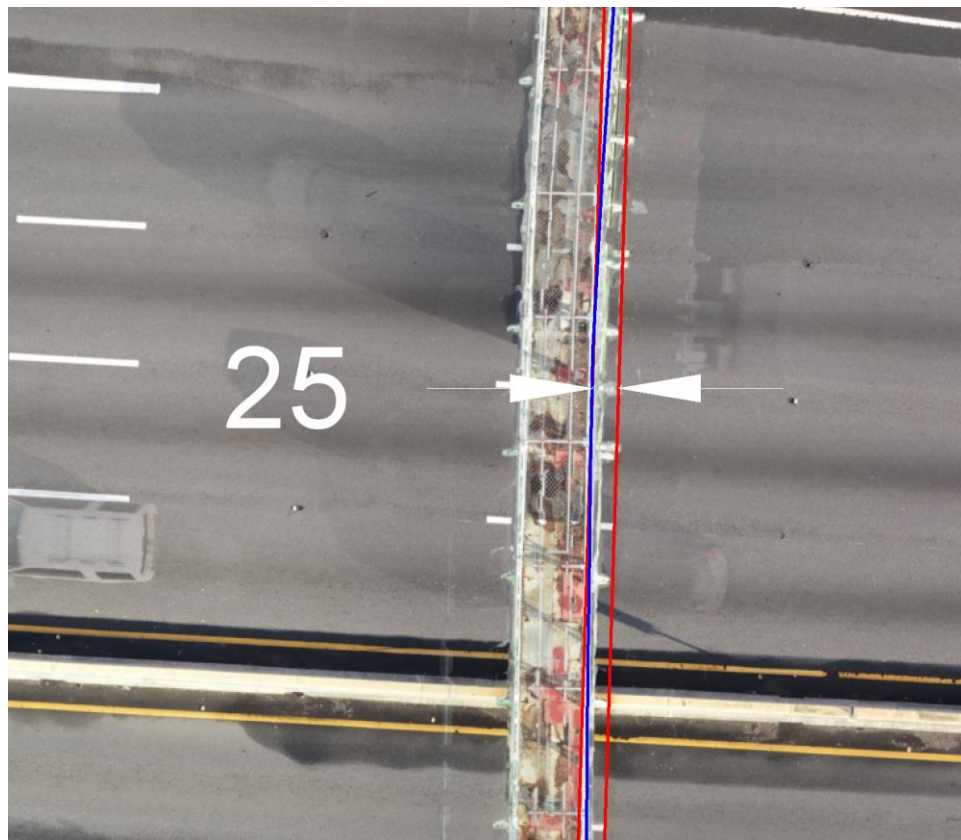
Figure 6.6: Bridge Maximum Plastic Deflection (in inches)
