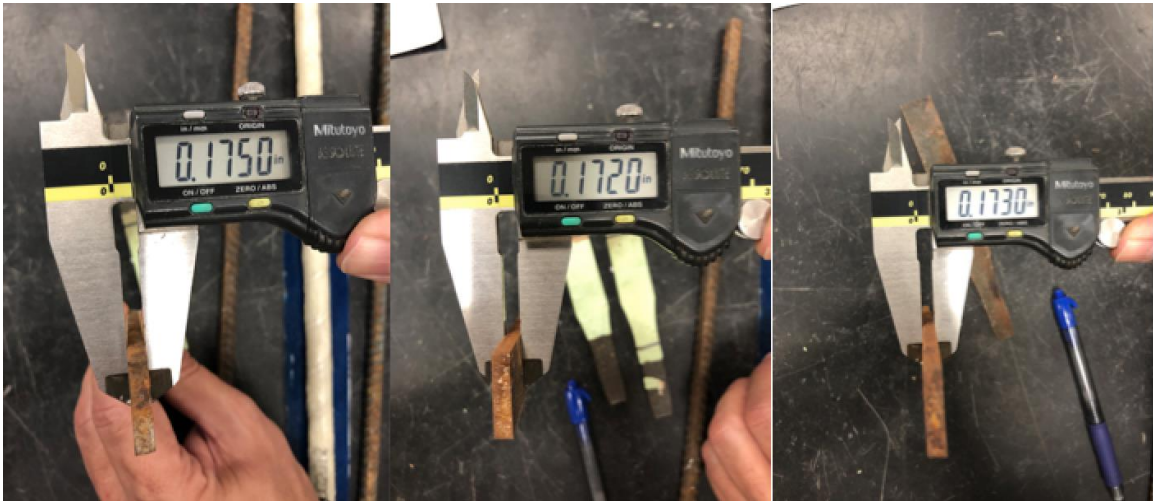
Figure 7.11: Measurement of Specimen Thickness
