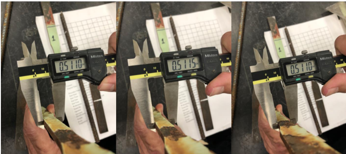
Figure 7.12: Measurement of Specimen Width
