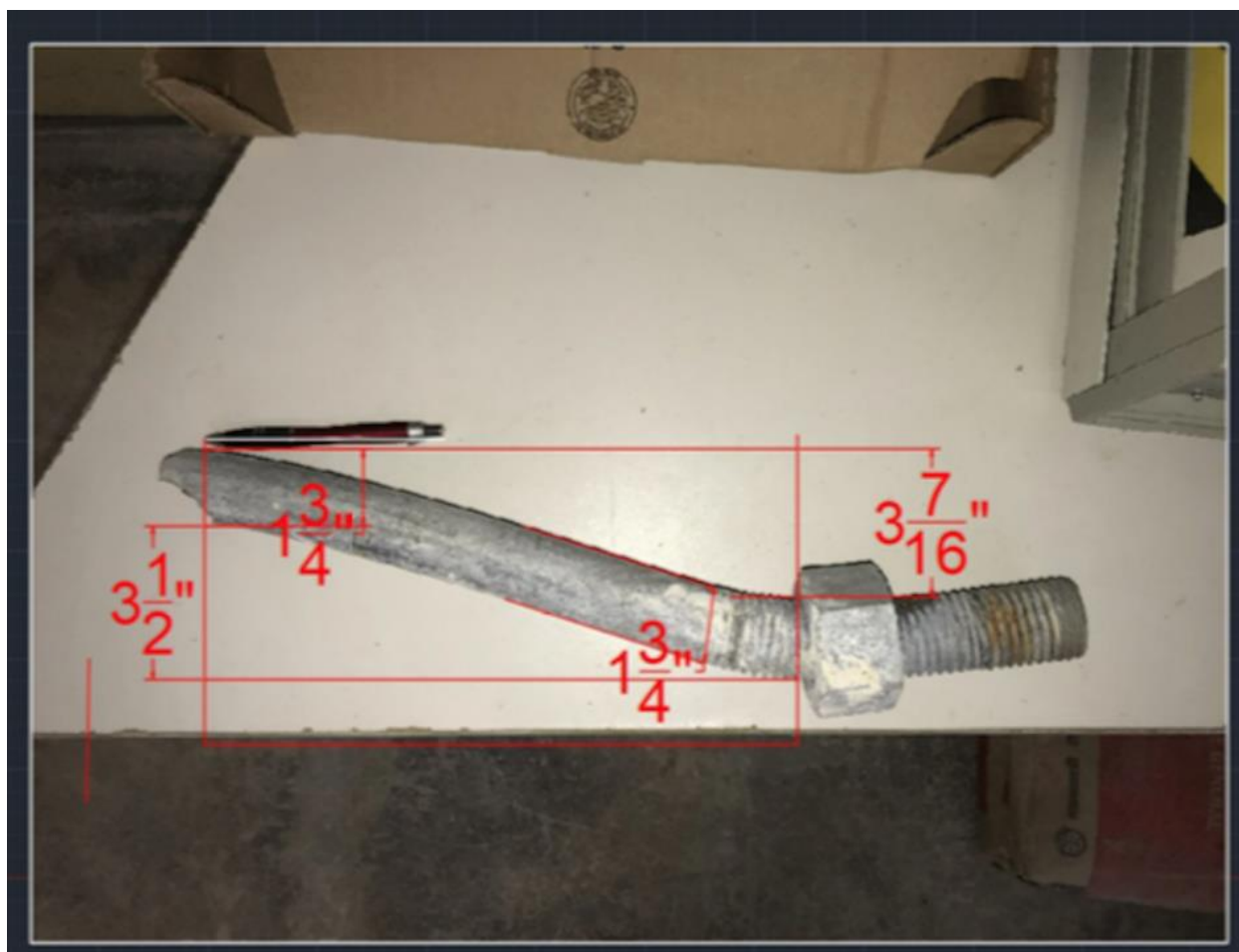
Figure 8-6: Anchor Bolt Sample with Plastic Deformations
