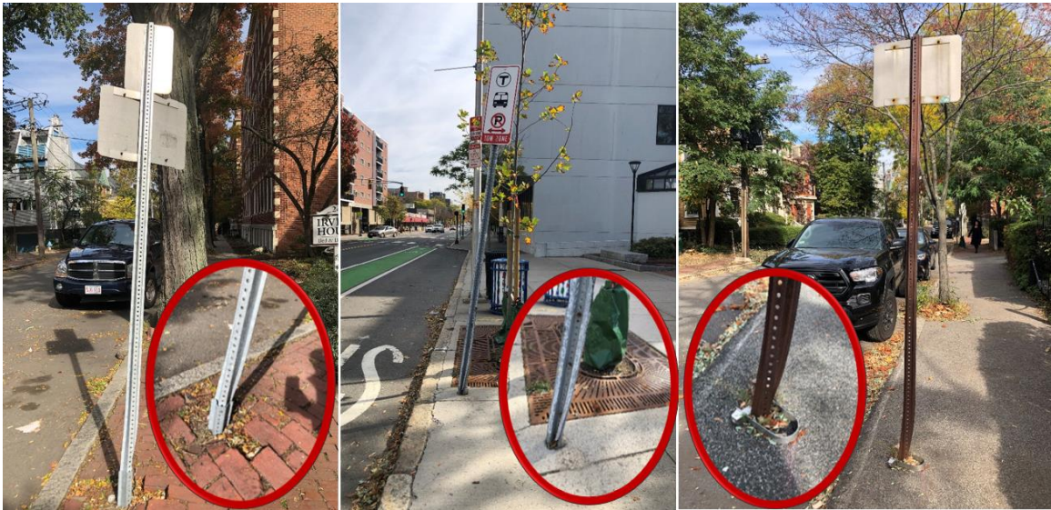
Figure 4.19: Permanent twisting deformation in U-channels in Cambridge, MA
