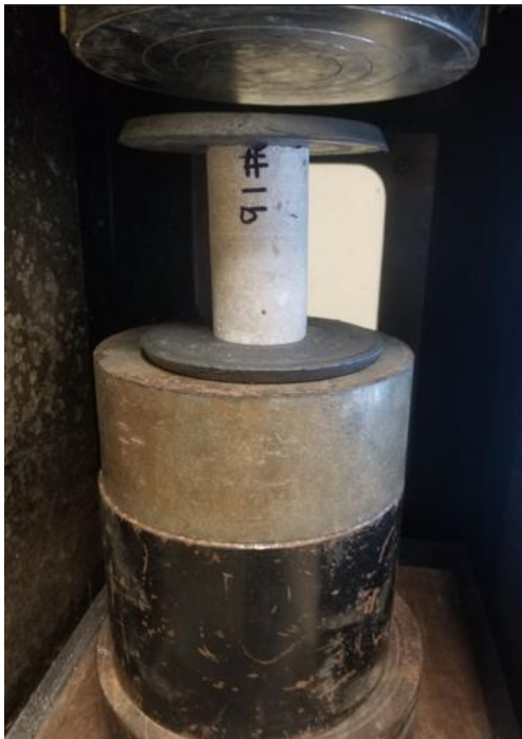
Figure 8-8 Example Mechanical Test to Core Obtained Concrete Cylinders
