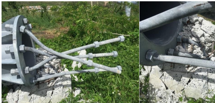
Figure 5-47: Photo on Cantilever Sign Foundation Structural Failure at P-105; Collapsed Post Presented Large Deflections and Bending on the Plastic Range and Shear Fracture of the Anchor Elements
