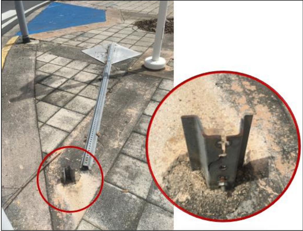
Figure 4.6: Example of tear-out failure
