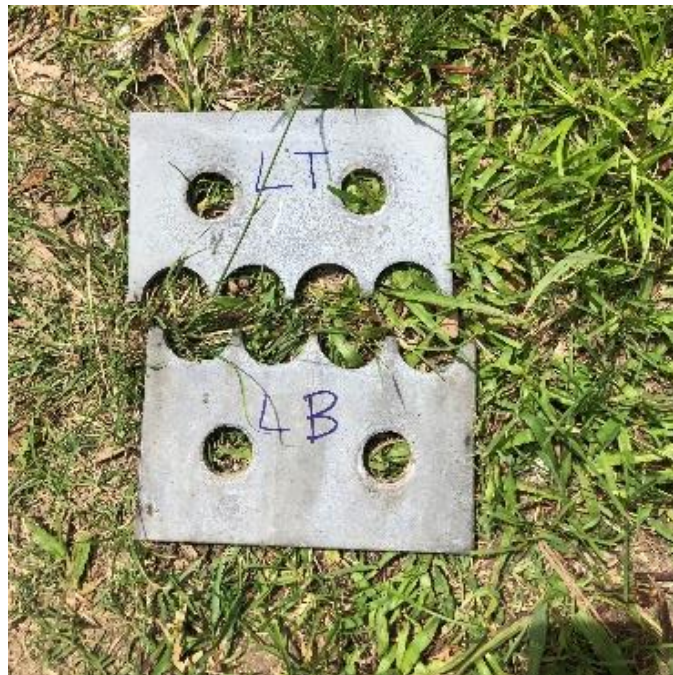
Figure 5.5 Fuse plate retrieved from Case 1
