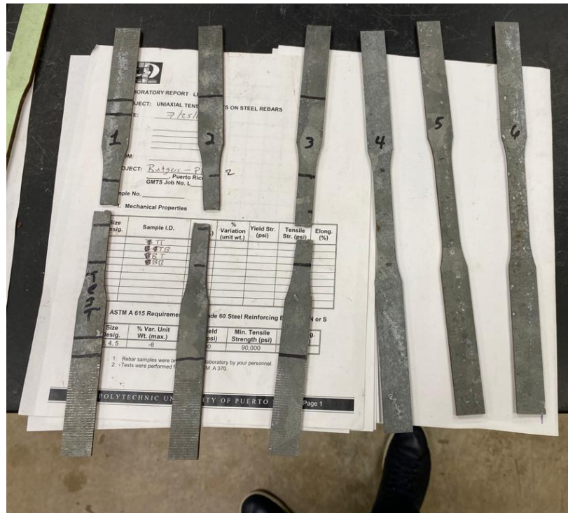
Figure 6.8: Specimens extracted from U-channel post
