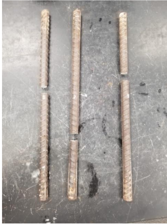
Figure 8-3: Reinforcing steel specimen after test was conducted
