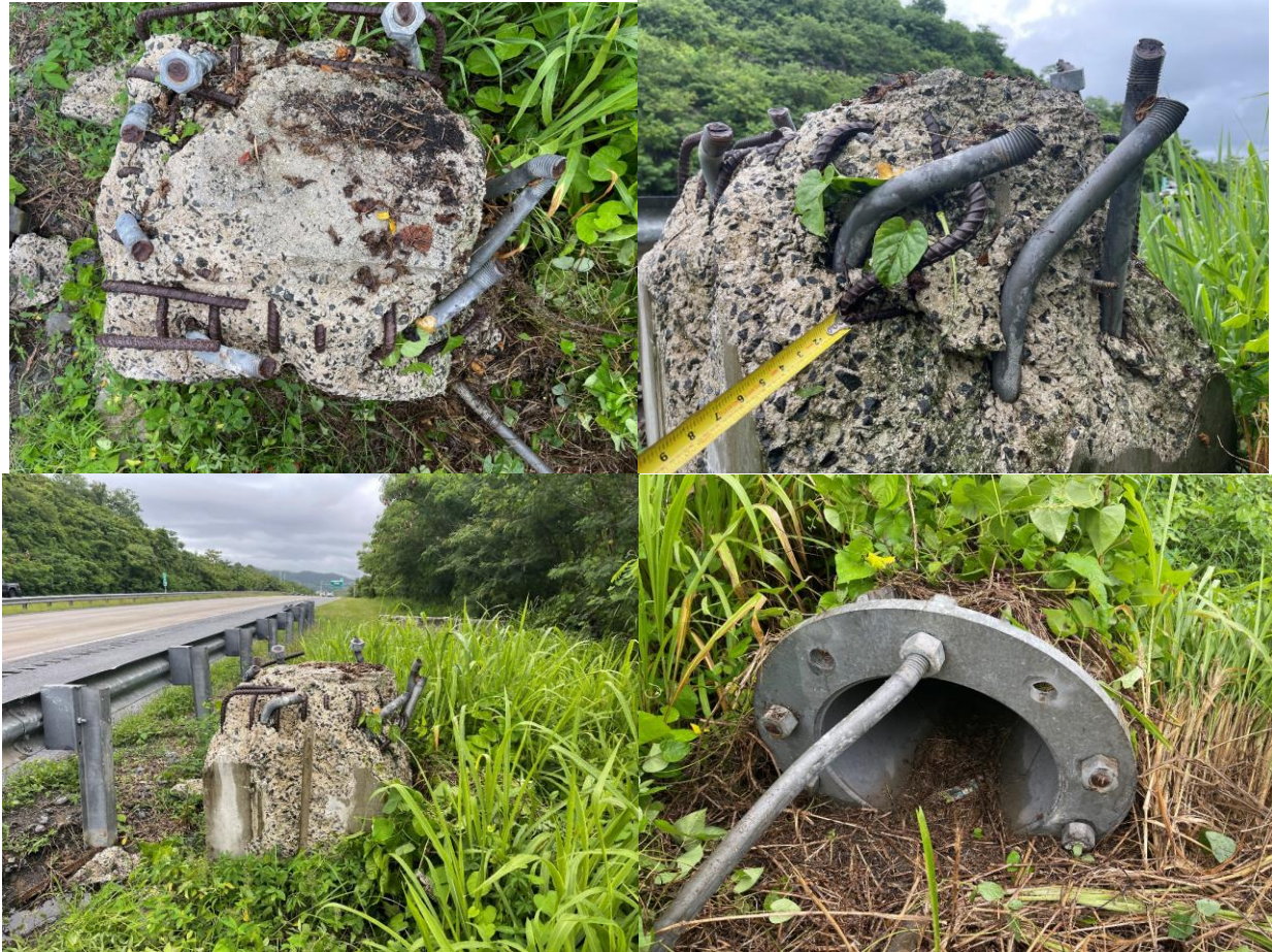
Figure 5-43: Photos of Cantilever Traffic Sign Foundation Structural Failure to the Pedestal at P-46; with Large Deflections and Bending on the Plastic Range and Shear Fracture of the Anchor Elements, and Fractures and Detachments of the Concrete
