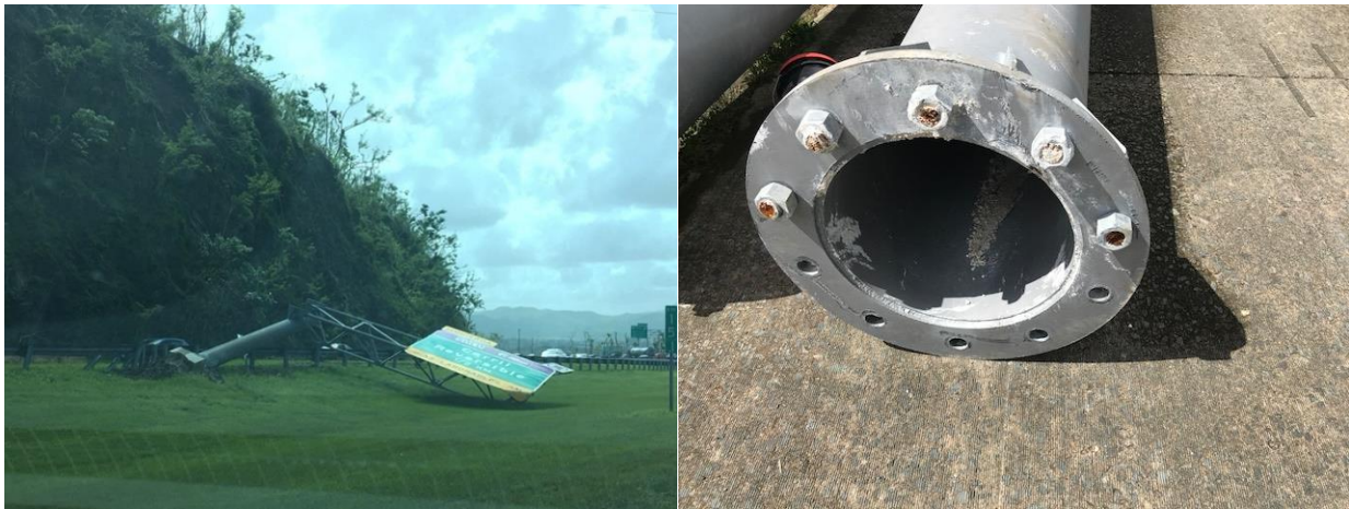
Figure 5-29: Photos of Cantilever Traffic Sign Overturning Foundation Failure and Anchor Bolts Shear/Tension Failure at P-52. Location: 18°11'7.35"N; 66° 3'17.55"W
