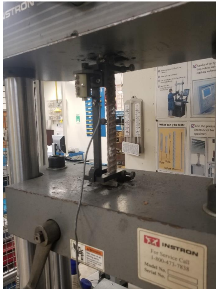
Figure 8-2: Tension Test of Longitudinal Rebar Specimen (Bar Size # 6, Diameter 0.097 Inches.)
