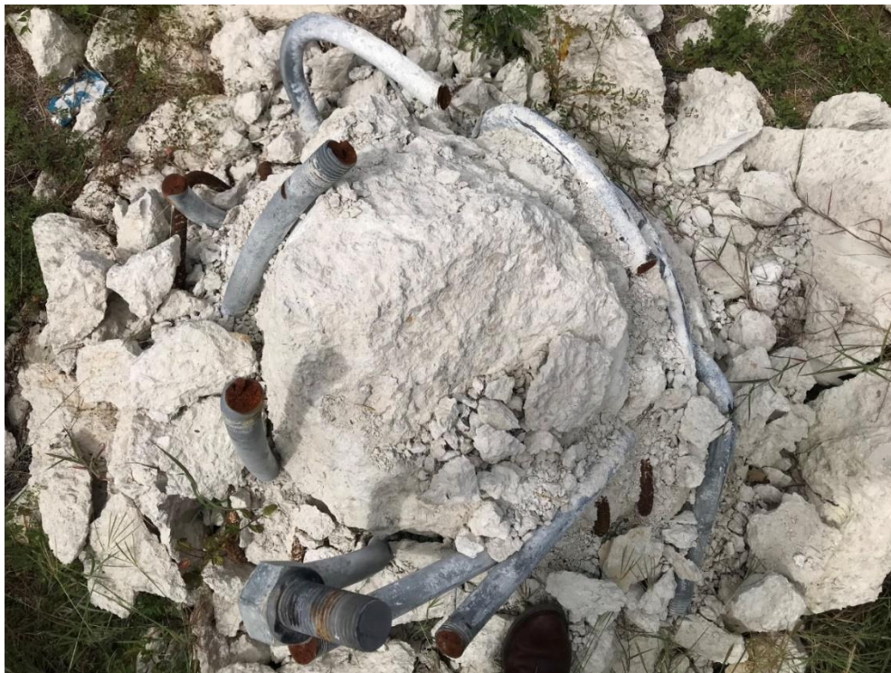
Figure 6-10: Large Deflections of Anchor Bolts due to Lack of Lateral Confinement (Sign P-12)
