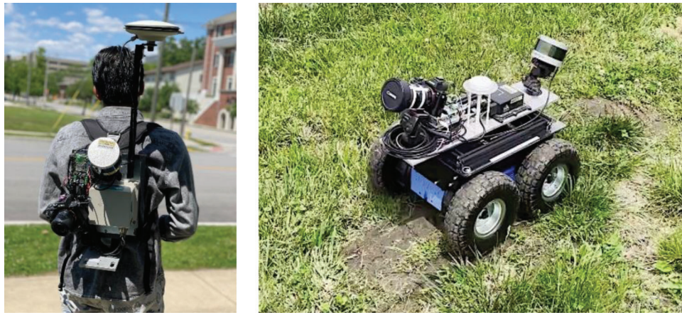
Figure 3.2 Backpack and UGV-based mobile mapping platforms.
