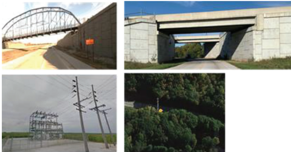
Figure 1.1 Examples of environmental factors that will impact the quality of the GNSS trajectory (from left to right): steel overpass, concrete bridge overpass, electromagnetic interference, and heavy canopy cover.
