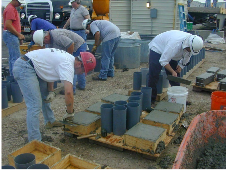
Figure 1.2 Casting of the 12"×12" Specimens
