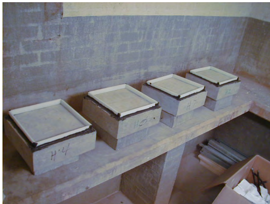
Figure 4.4 Construction of Dams for the Houston Samples
