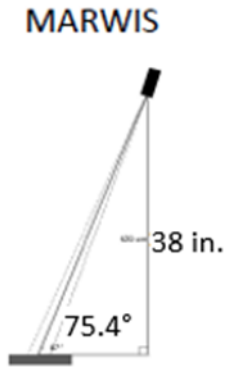
Figure 8. Recommended mounting height and angle for the MARWIS
