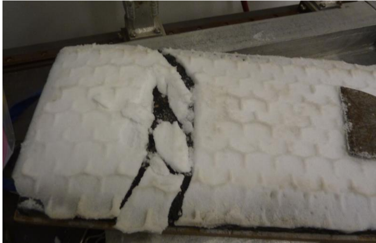
Figure 14. Trafficked snow scraped off the asphalt pavement sample
