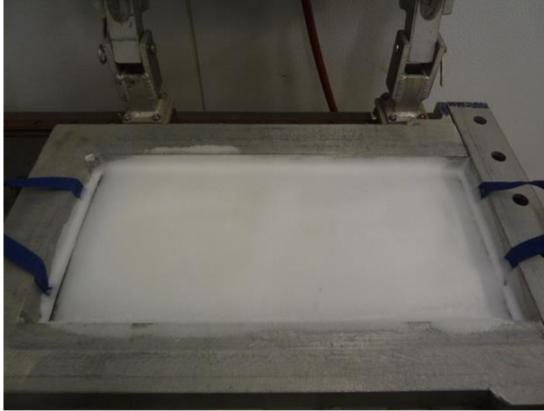
Figure 12. Pavement sample with compacted snow in the compaction machine
