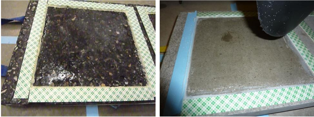
Figure 10. Asphalt and concrete samples with the 7 by 7 in. silicon dam for water depth/ice depth measurements
