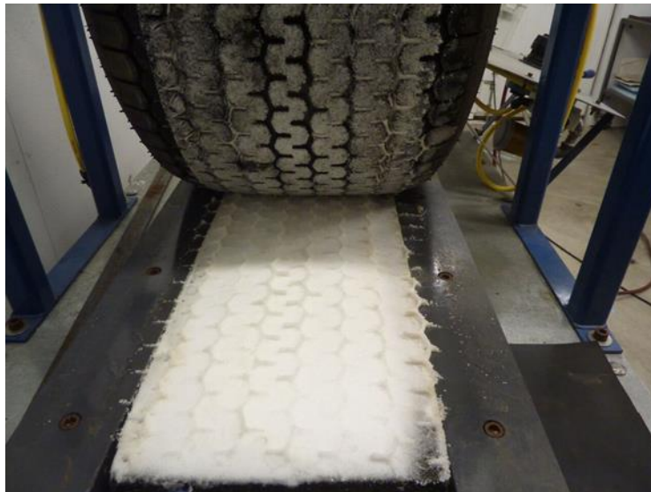
Figure 13. Trafficking of snow on an asphalt pavement sample
