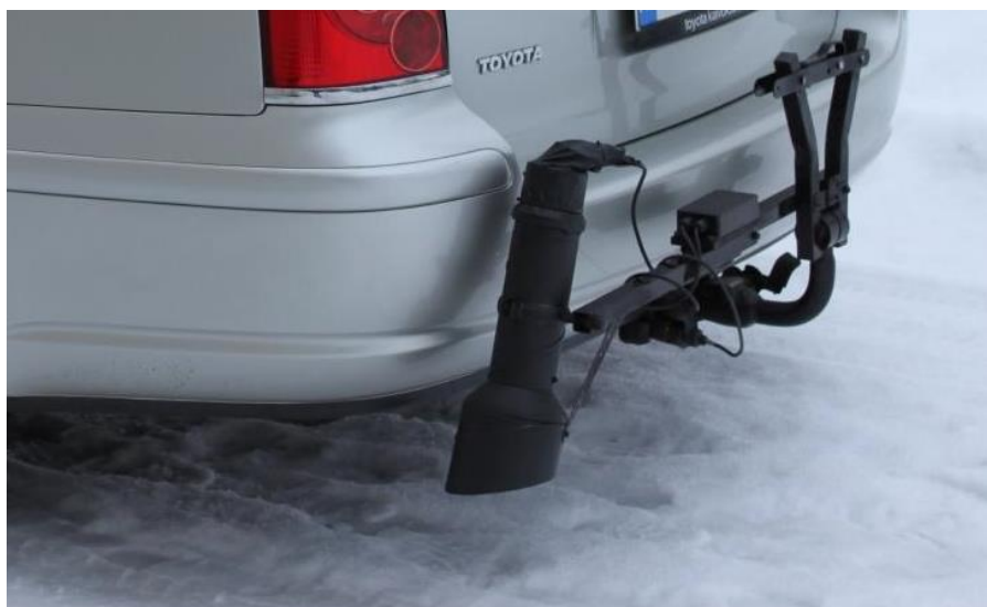
Figure 3. Teconer RCM411 mounted on the rear bumper of passenger vehicle
