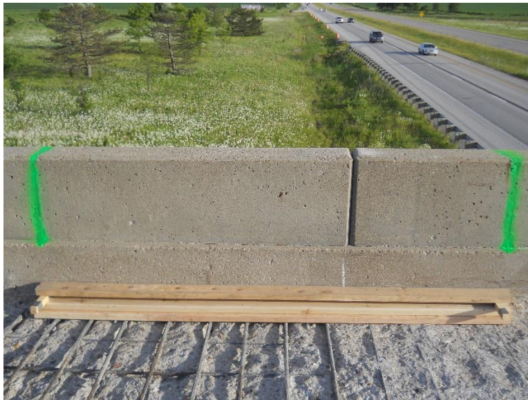
Figure 36. Configuration of material used to elevate the antenna to mimic the 2012 inspection location
