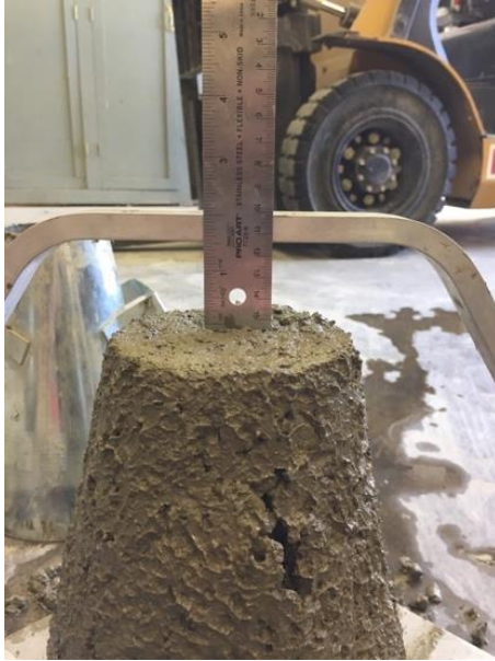
(a) Slump Test
