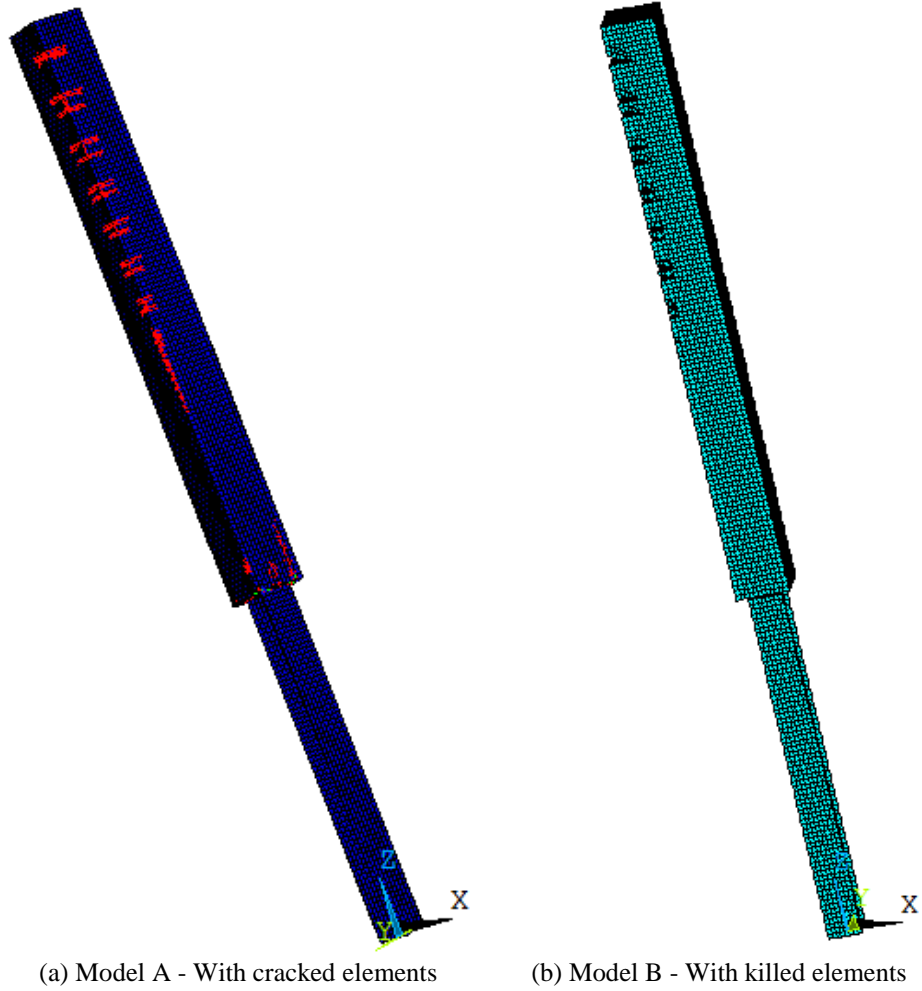
Figure 3.12 FE model with different crack modeling techniques
