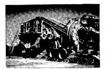
13. For large sized RAP, a primary jaw crusher of sufficient size, 30 x 42 inch minimum, is required. For smaller RAP, crushing may be accomplished with a secondary crusher. RAP from thick asphalt pavements usually requires both.
