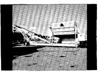
39. Conventional conveying equipment can be used to feed RAP into either batch or drum mixer plants. RAP bins should have relatively small capacity with steep sides and wide, long bottom openings to allow for easy discharge and minimal sticking problems. The RAP should be dribbled into the bin, since a unit drop could compact the RAP. Vibrators should not be used on this bin since they encourage compaction of the RAP.
