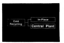
31. Central plants can also be used for cold-mix asphalt recycling. Their advantages include better quality control, easier proportioning and blending of new aggregate, and higher production rates. However, there are added hauling costs and the potential for increased traffic disruption. Central plants may be economical in locations where a plant is already available.
