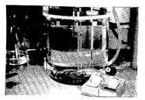
43. Extraction and recovery tests should be performed on each field sample to determine its asphalt content. The recovered asphalt should be tested for penetration and viscosity (pictured). Extracted aggregates should be tested for gradation and quality. Any RAM and new aggregates should be tested for gradation, fractured faces and cleanliness.
