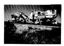
20. In this view, a portable crusher has been attached to a cold milling machine. The milled RAP is conveyed to the top of the portable crusher. After crushing, the recycled mix is deposited in a windrow behind the crusher.
