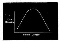
35. Achieving proper fluids content, modifiers and water, is a critical part of the laydown and compaction process. Some amount of fluids are required for compaction. They also help to prevent sticking to the screed and reduce tearing of the surface.
