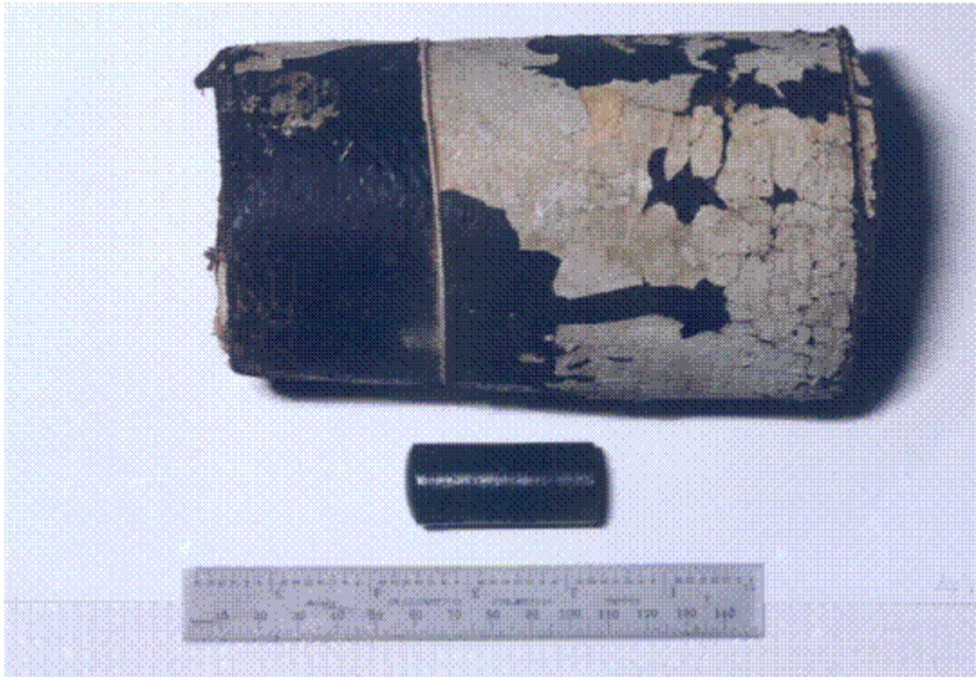
Figure 2. Volume reductions achievable with the caustic-only or caustic-acid-caustic dissolution methodologies coupled with Joule Heated Ceramic Melting (JHCM).
