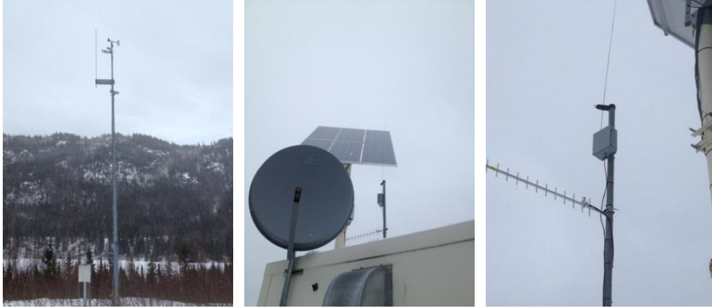
Figure 6. Weather sensors and communications equipment at remote RWIS site in Alaska, from left to right: meteorological tower, satellite dish, and communications antenna
