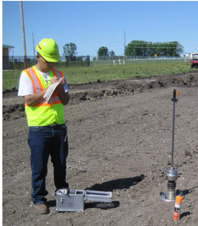
Figure 12. Zorn light weight deflectometer
