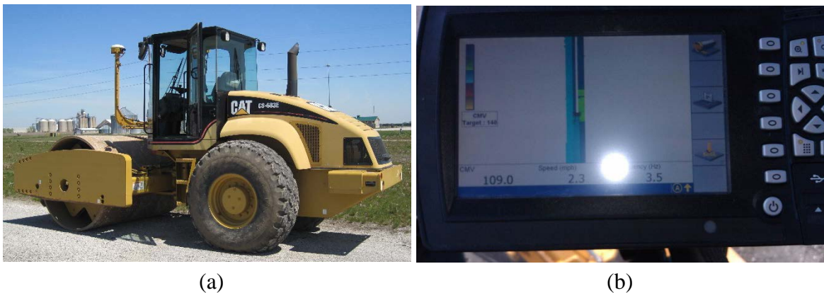
Figure 16. (a) Caterpillar CS683 vibratory smooth drum roller, (b) Caterpillar on-board display monitor
