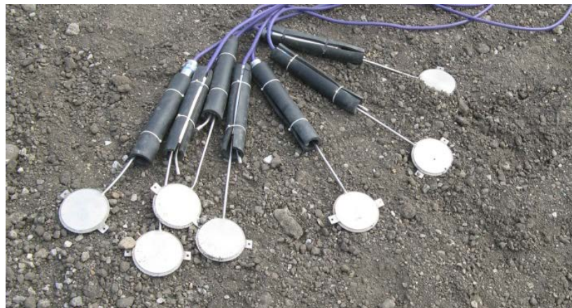
Figure 20. Earth pressure cells (EPC)
