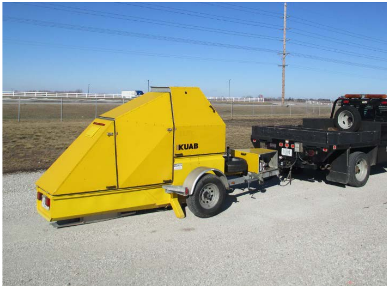
Figure 13. Kuab falling weight deflectometer
