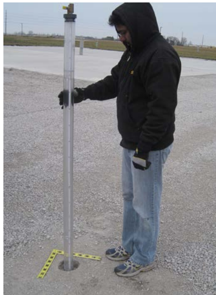
Figure 23. In situ MPT setup for determination of saturated hydraulic conductivity
