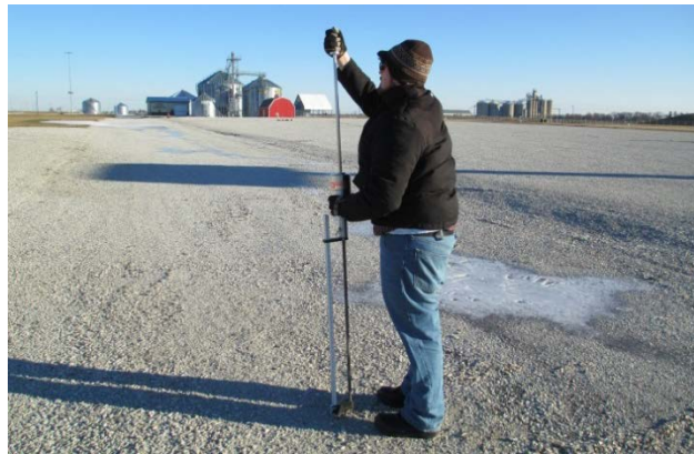
Figure 14. Dynamic cone penetrometer
