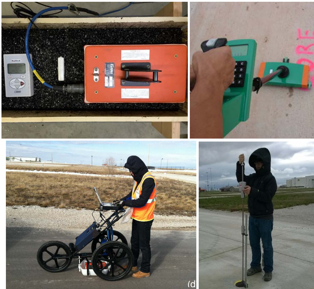
Figure 262. (a) Test setup using GS3 sensor and GPR antenna in laboratory box study; (b) MIT gauge; (c) GPR setup with a scanning survey wheel setup in situ; and (d) DCP testing of the foundation layer through a pavement core
