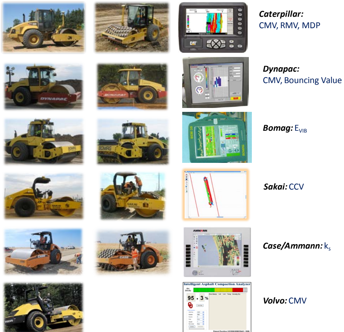
Figure 10. Pictures of various roller manufacturers, roller configurations, and display software's with RICM technology (note that this does not represent a complete list)
