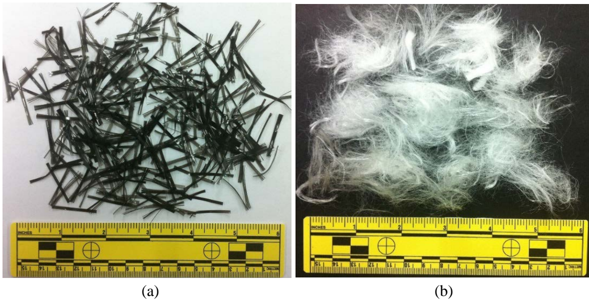
Figure 27. (a) Black MF-PP fibers, and (b) white fibrillated PP fibers
