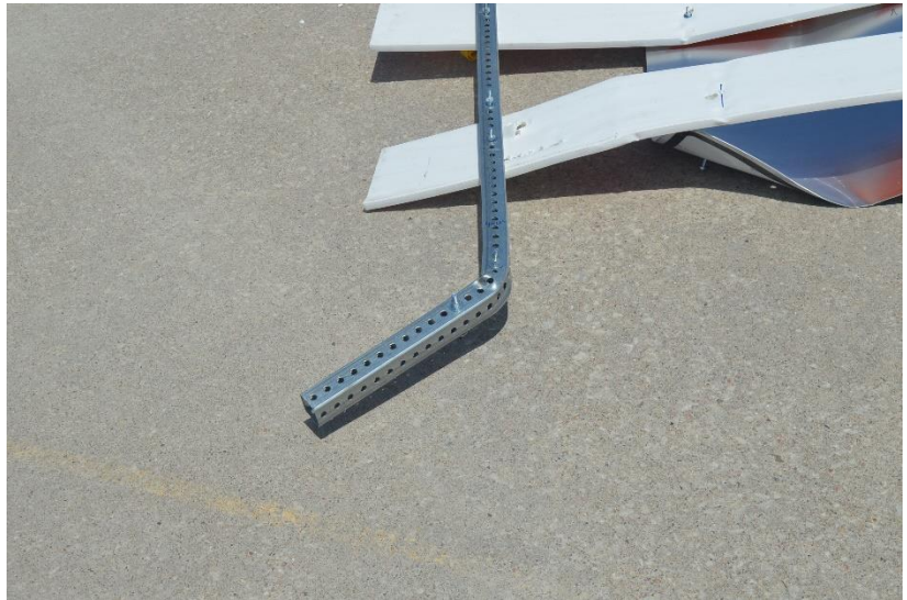
Figure 64. System Damage –Test No. WZNP-1, System B
