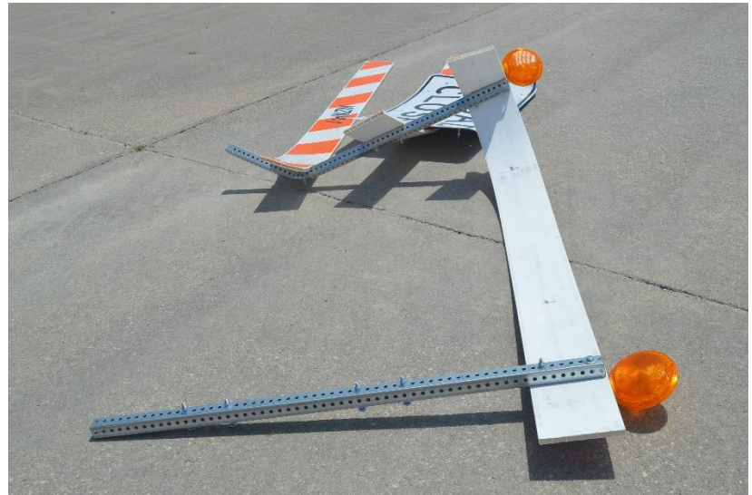
Figure 63. System Damage –Test No. WZNP-1, System A
