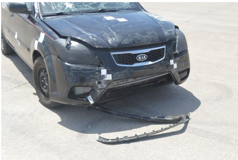
Figure 66. Vehicle Damage, Test No. WZNP-1
