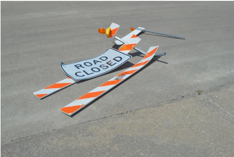
Figure 63. System Damage –Test No. WZNP-1, System A
