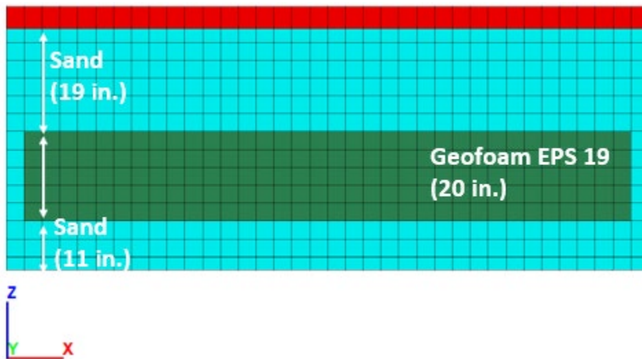
Figure C15. A cross-section in X direction for scenario 8-Geofoam EPS 19 (20 in. thick in Z direction).
