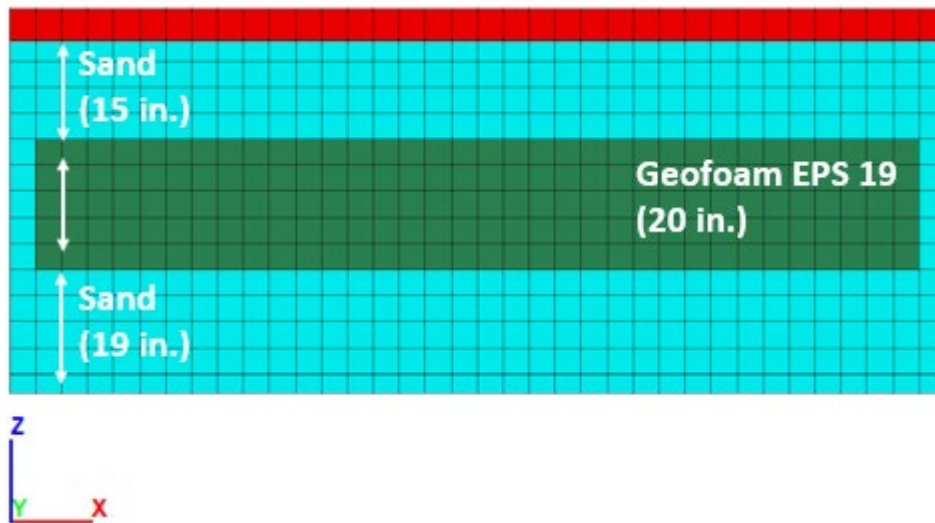
Figure C17. A cross-section in X direction for scenario 9-Geofoam EPS 19 (20 in. thick in Z direction).
