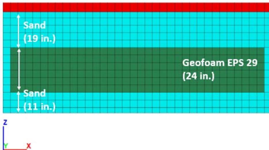
Figure C37. A cross-section in X direction for scenario 19-Geofoam EPS 29 (24 in. thick in Z direction).
