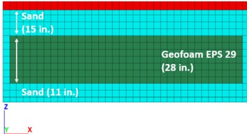
Figure C49. A cross-section in X direction for scenario 25-Geofoam EPS 29 (28 in. thick in Z direction).
