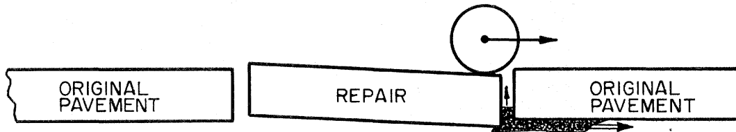
c) Wheel Approaches Repair Leave Joint, Pushing Excess Moisture Ahead
