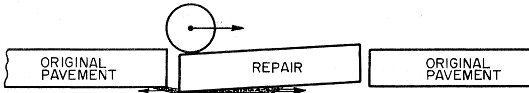
a) Moisture is Squeezed Forward by Approaching Wheel Load
