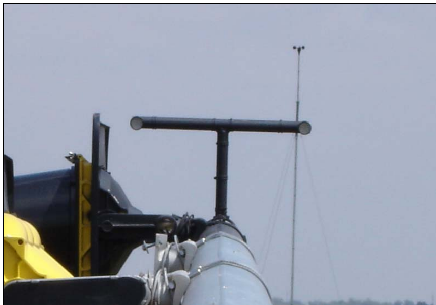
Figure 3.9 Infrared Target as Viewed from Top of Pole
