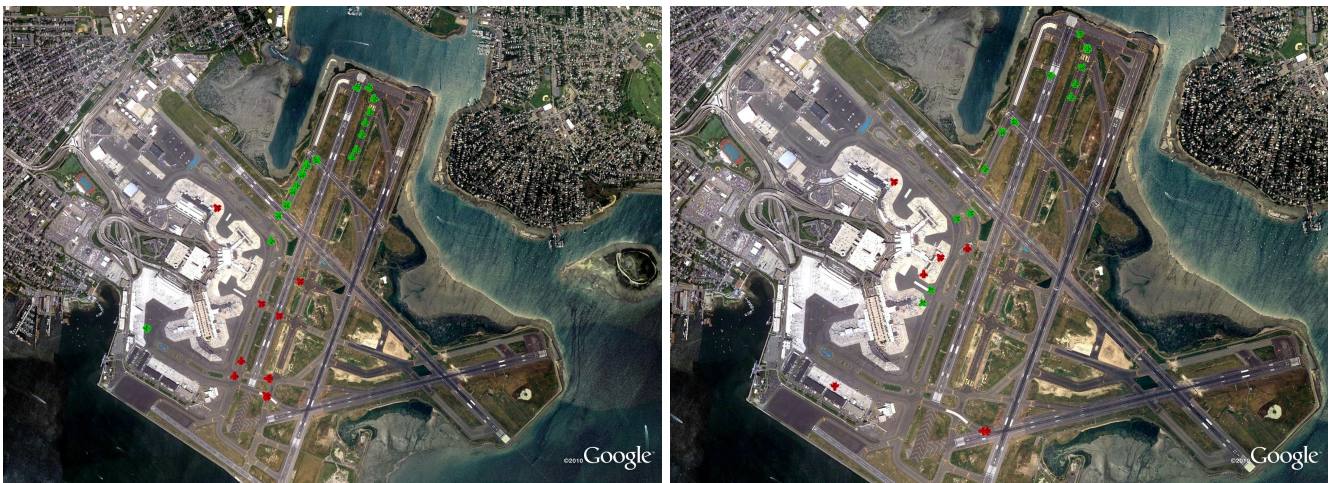
Fig. 10: Snapshots of the airport surface, (left) before gate-holds started, and (right) during gate-holding. Departing aircraft are shown in green, and arrivals in red. We note that the line of 15 departures between the ramp area and the departure runway prior to commencement of pushback rate control reduces to 8 departures with gate-holds. The white area on the taxiway near the top of the images indicates the closed portion of taxiway “November”.
