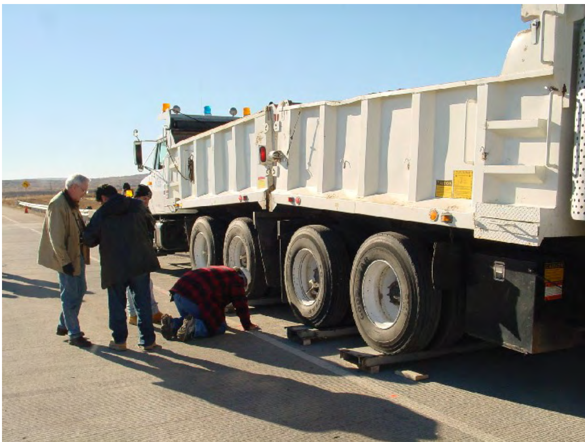
Figure 4.3 Crack Measuring with TxDOT Dump Trucks in a Back-to-back Load Case Photograph: Courtesy of Alvin Gutierrez, FHWA
