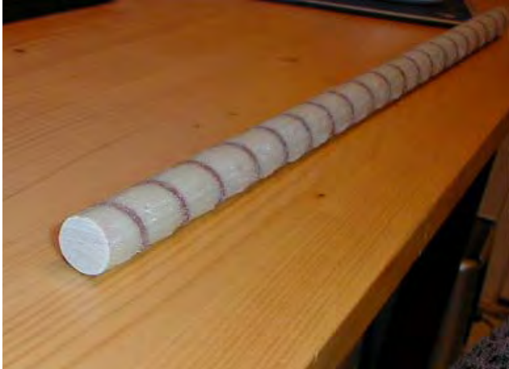
Figure 1.3 Hughes Brothers Aslan 100 GFRP Bar Sample
