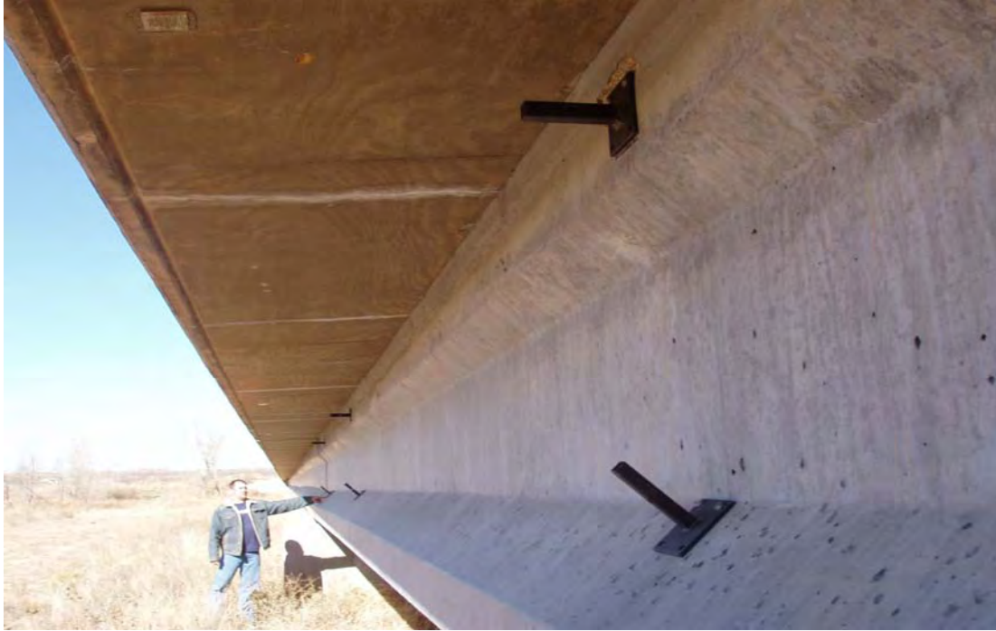
Figure D.1 LVDT Mounting Brackets on Span 6
