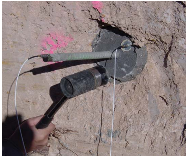
Figure 4 Hitting the Grout Column Head with 0.2-lb Hammer
