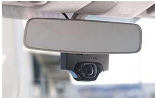
Figure 1. DriveCam Event-Triggered Video Data Recorder
