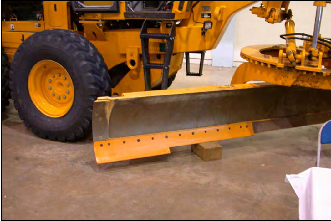
FIG. 7.6 Motor Grader Blade Extension for Reshaping Pavement Edges, Waco District (refer to Waco District for detailed fabrication plans)
