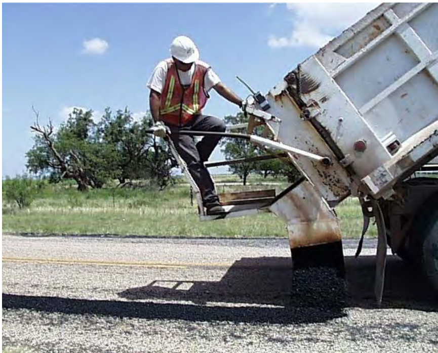
FIG. 7.14 Side Discharge Chute with Operator Platform and Material Flow Regulation Lever, Abilene District ( Photo courtesy of Jones County Maintenance )
