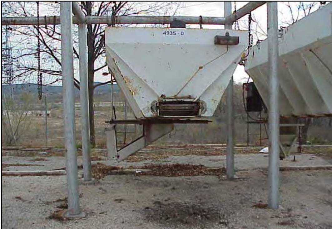
FIG. 7.19 Modified V-Box Side Discharge Spreader: Front View, San Angelo District (see San Angelo District Profile, Photo 19)
