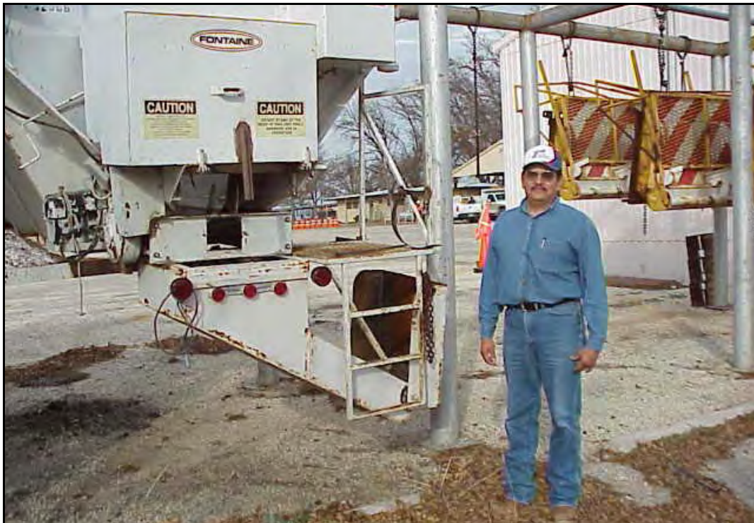
FIG. 7.17 Modified V-Box Side Discharge Spreader: End View, San Angelo District (see San Angelo District Profile, Photo 16)
