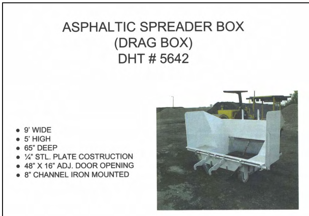
FIG. 7.10 Drag Box; Tow-Behind, Used for Delivering Windrow of Material to the Center of Pavement, Pharr District
