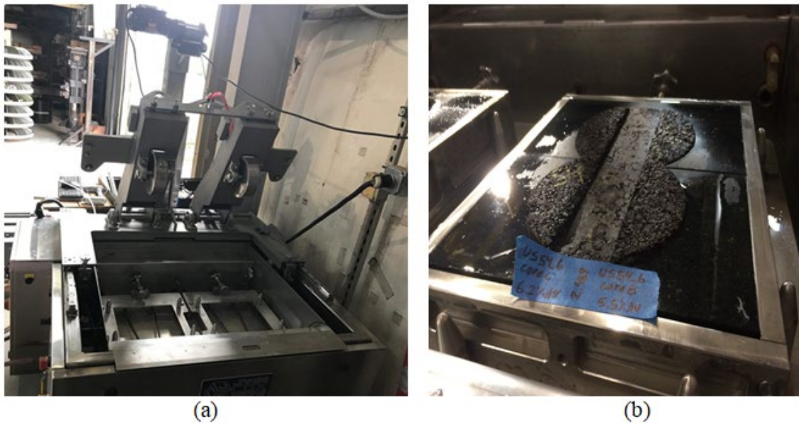
Figure 3-9. Hamburg Wheel Tracking device: a) Test device b) mixtures after test
