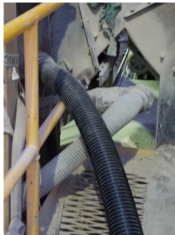
Figure 6-3. Connection of fiber and ECR-GTR hoses at similar location near bottom of drier drum
