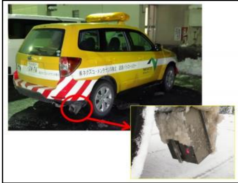
Figure 8. The installation of Yamada-Giken mobile salinity sensor
