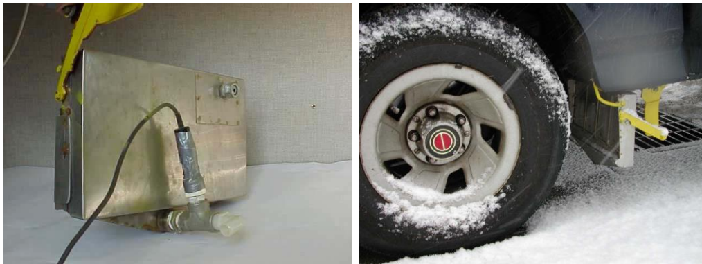
Figure 1. Portable salinity sensor deicer collection box (left) and on-vehicle mounting (right)
