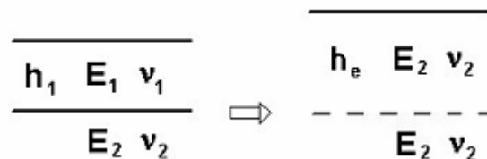
Figure 70. Odemark's transformation of a layered system, from ELMOD QuickStart Manual [Dynatest International, 2010].
