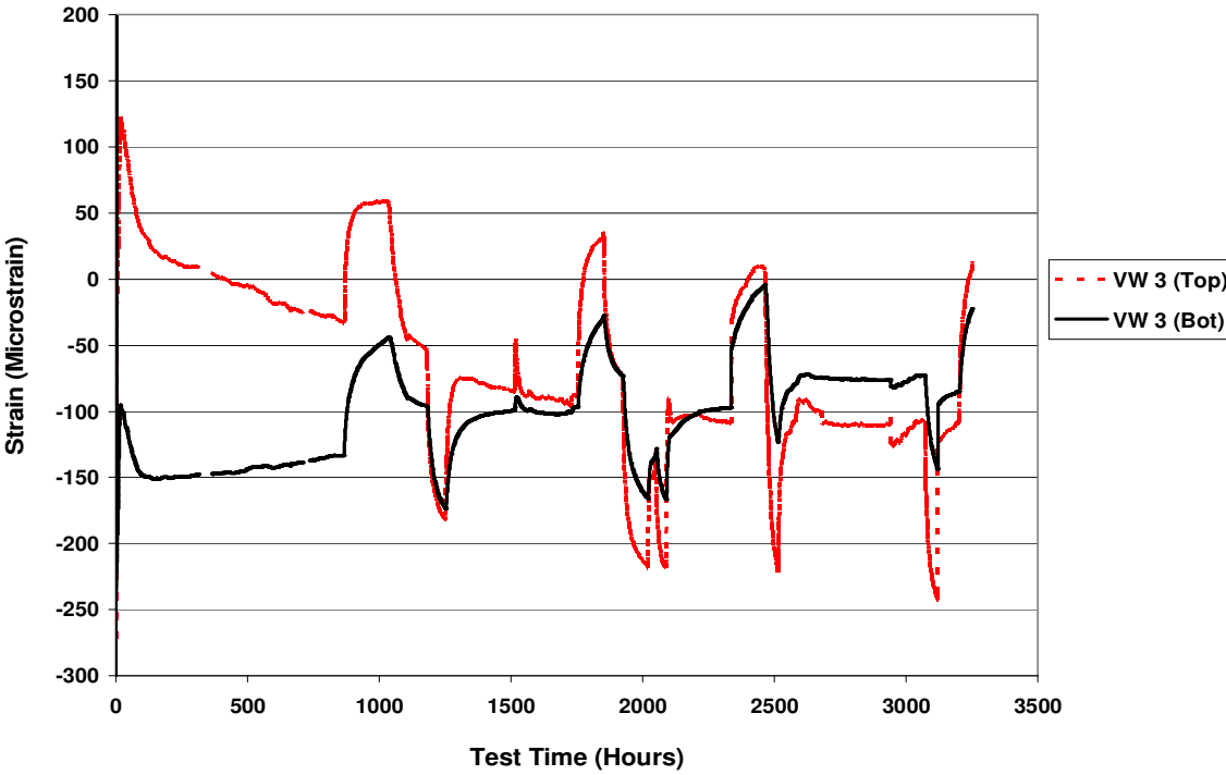
Figure 16. Top and Bottom Strain Development at Vibrating Wire Strain Gauge Location # 3. [Sargand and Abdalla, 2006]
