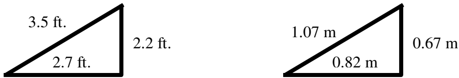
Figure 34. Extent of upward curling along the diagonal (left in English units, right in metric units).
