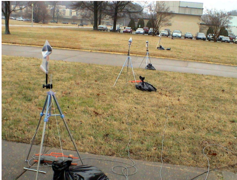
Figure 5: Long view of exterior microphones set up outside Bldg. 1208. Microphones shown were at distances 4, 9, 14, 25, and 53 m.
