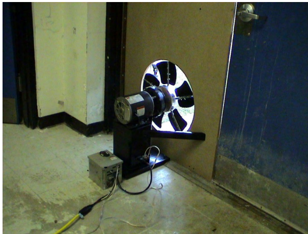
Figure 4: Interior and exterior views of rotary subwoofer installed in baffled exterior door. Interior view shows close up of fans of the rotary subwoofer device. Exterior view shows two of the microphones placed closest to the source, protected from rainy conditions, for monitoring resulting signatures.
