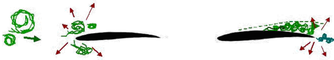
Figure 19: Noise Producing Turbulence over a Wing [Ref. 74]
