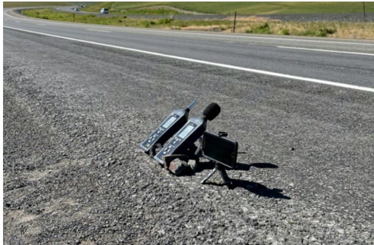
Figure 3.2 Sound Meter Field Setup (Along US-95)
