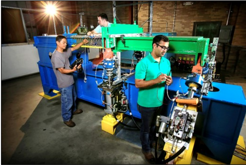
Figure 9. Engineers calibrate the ABST fixture to test an aircraft structural component. Source: Michael Gross.
