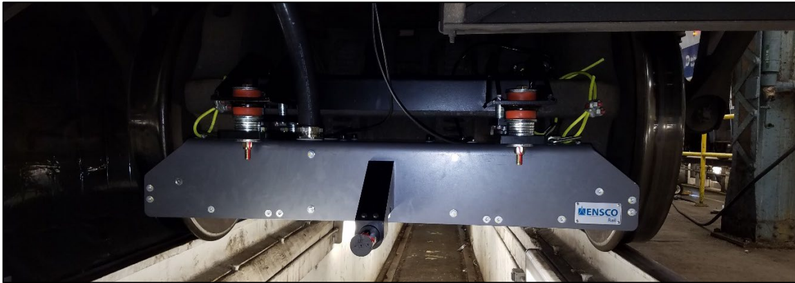
Figure 7. ATGMS installed on rail car operated by Metro North Railroad.
