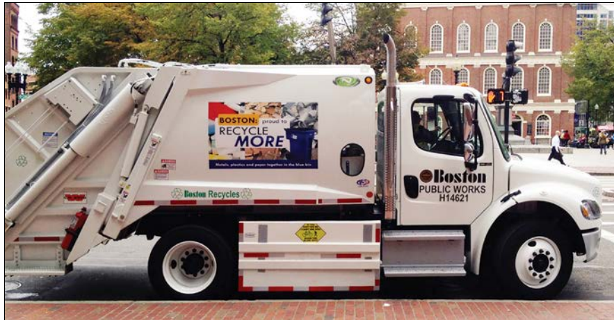
Figure 2 Side guards help keep pedestrians and bicyclists from falling between axles. Source: City of Boston.
