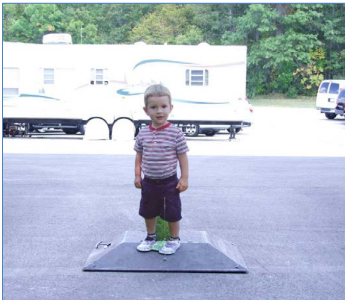
Figure 5 Photo of Programmable Robotic Child Obstacle as Presented in NHTSA Research Evaluating the Effectiveness of Rear Visibility Crash Avoidance Aids for Drivers
