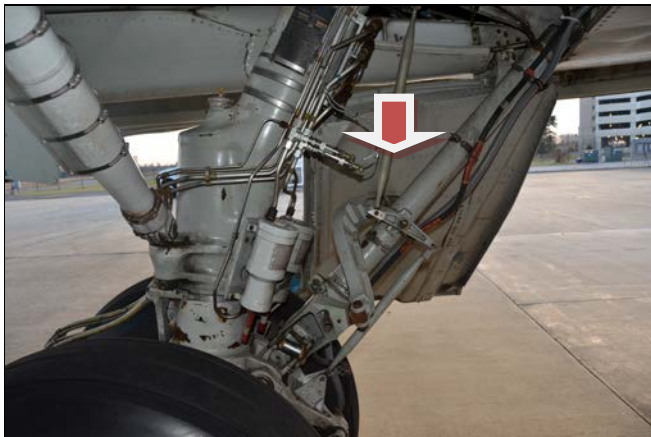
Figure 8 Image showing pressure transducers
