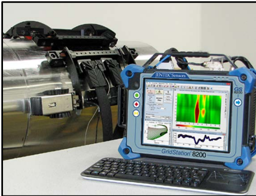
Figure 3 MWM Corrosion, Mechanical Damage and SCC imaging courtesy of JENTEK
