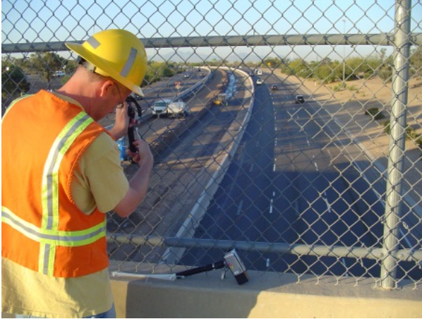
Figure 11 Volpe Center team is shown measuring highway noise (Volpe Center photo).
