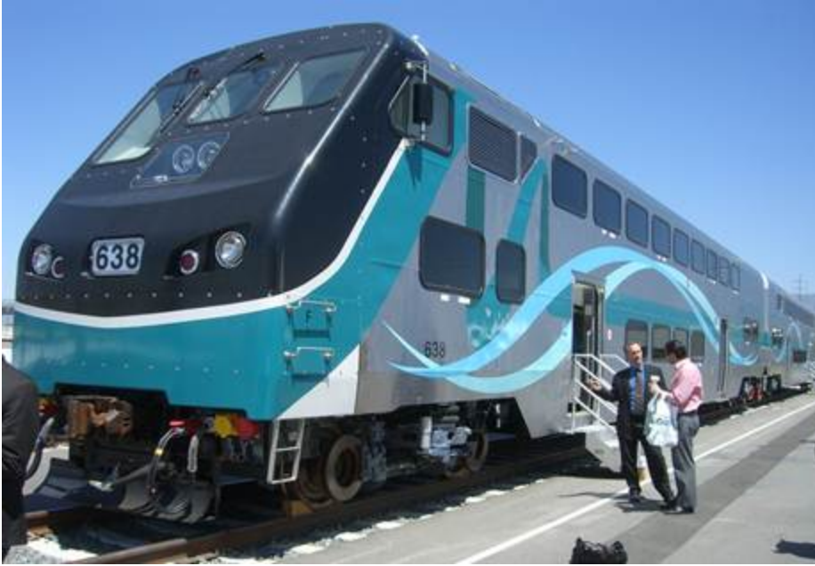
Figure 3 A new Los Angeles Metrolink cab car using the safer Volpe Center design for improved passenger protection in crashes.
