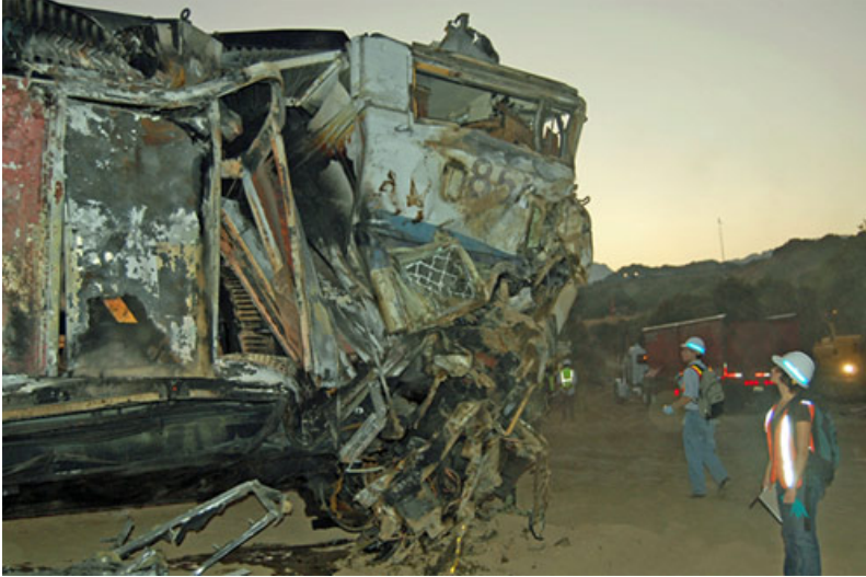
Figure 2 Volpe crashworthiness experts investigated the lead locomotive of the Chatsworth, CA rail accident ( Volpe Center Photo )
