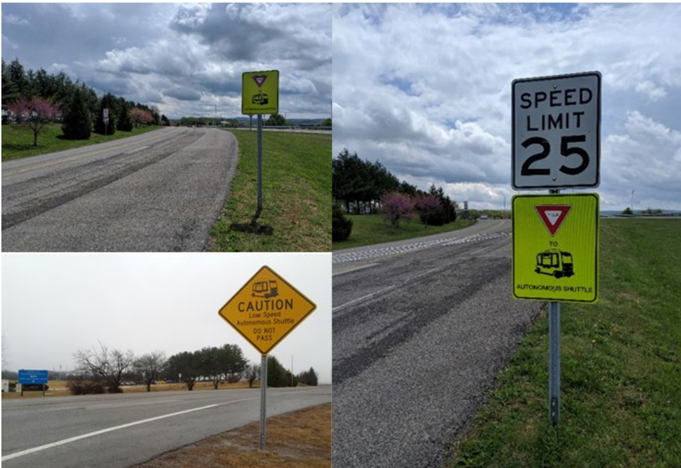
Figure 8. Photographs of the various signs that were installed along the LSAV's route to provide notification to the public traffic using the road.
